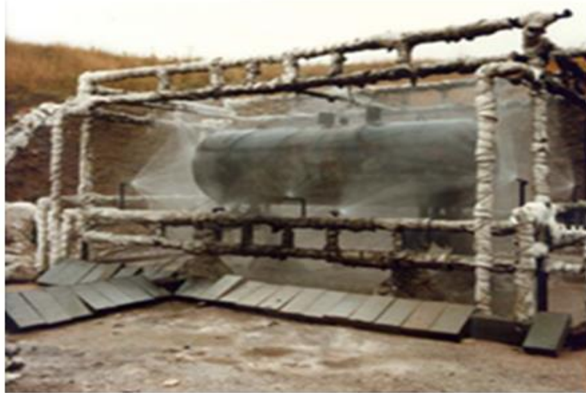
Figure 9: water sprinkler on the LPG tank (T Roberts, I Buckland and H Beckett, 2001)
