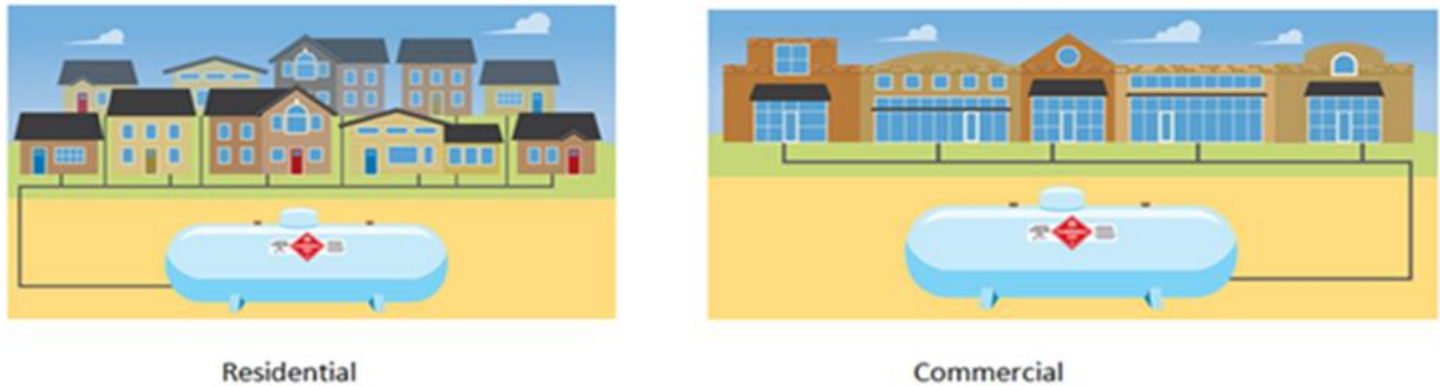
Figure2: LPG systems for use in residential and commercial buildings (National Academy of Sciences, 2018)
