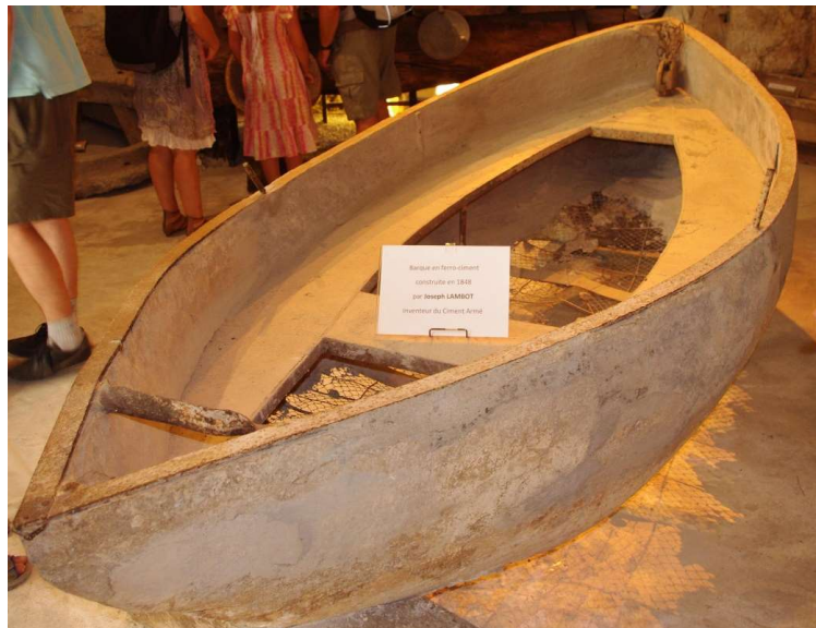
Fig.1. 2- This is a model of the ferrocement boat that Lambot built in 1856.
