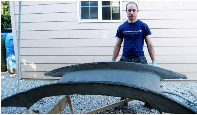
Fig.2. 19 -Spooner's deck bridge (covered with cement mortar ).
