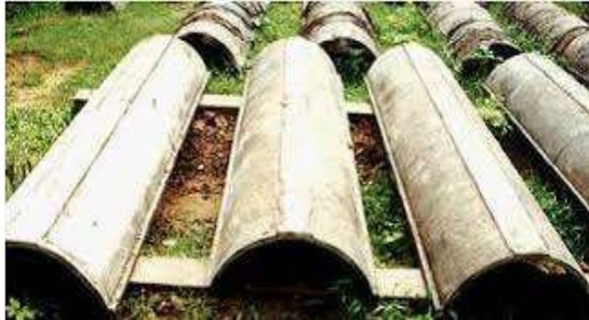
Fig.2. 8 - Precast ferrocement panels for roofing.
