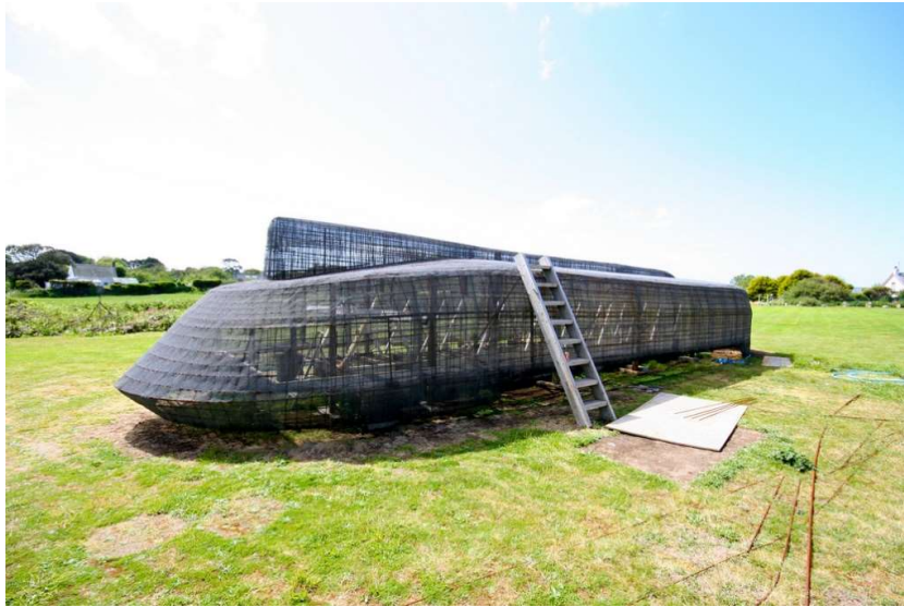
Fig.2. 1— A ferrocement house boat designed by (Ricky's Ferrocement Barge Co.) in Guernsey 2013 (under construction) .
