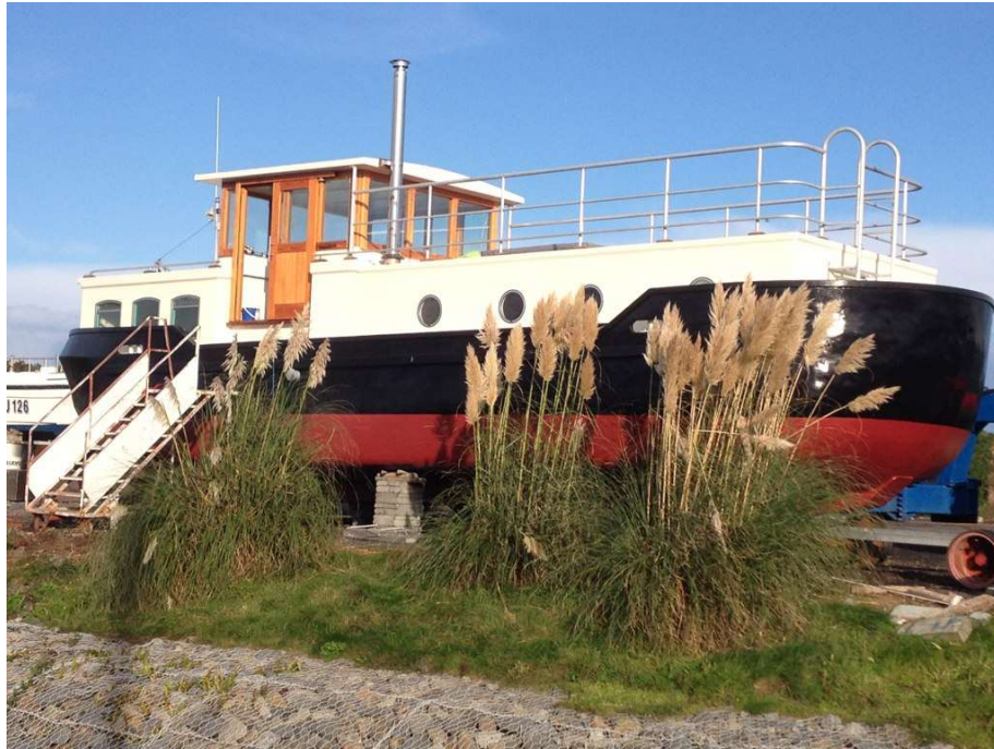
Fig.2. 2— A ferrocement boat designed by (Ricky's Ferrocement Barge Co.) in Guernsey 2013 (completed).
