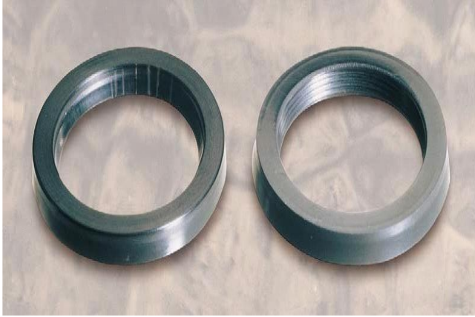
Figure 2-29 Contamination damage is apparent in this rod seal, where the serrations are worn completely away. The seal on the right is a new one, shown for comparison.
