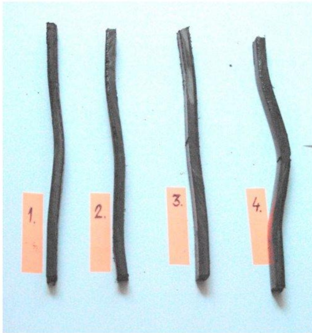
Figure 10. Compression test specimens.
