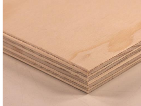
Figure 219, Plywood layer construction.
