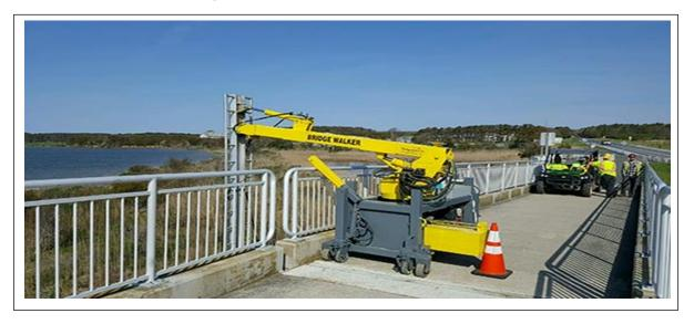
One of the biggest risks faced by bridge workers is falling from a higher level of a bridge to a lower one. This often happens because workers use the wrong equipment to access hard-to-reach sections of bridges. They retrofit equipment designed for other purposes or come up with temporary solutions to get to those areas.
