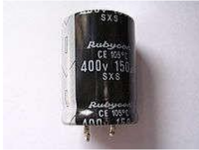
Figure 3.14: A typical electrolytic capacitor
