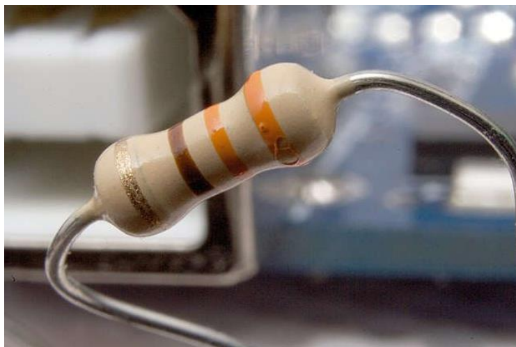
Figure 3.6: A typical axial-lead resistor
