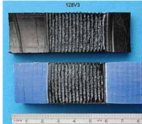
Fig.5. Fracture surface of ISO peel decohesion test specimen showing fully ductile failure through the plane of the heating wires
