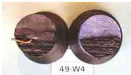
Fig.12. Fracture surface of tensile creep test specimen showing a mixed failure mode
