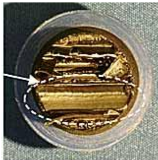
Fig.9. Fracture surface of tensile creep test specimen containing a void
