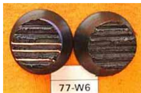
Fig.10. Fracture surface of tensile creep test specimen through the plane of the heating wires
