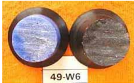
Fig.11. Fracture surface of tensile creep test specimen through the weld interface
