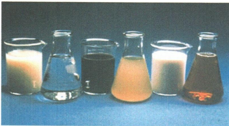
Fig.(1) Liquid admixtures, from left to right: antiwashout admixture, shrinkage reducer, water reducer, foaming agent, corrosion inhibitor, and air-entraining admixture.
