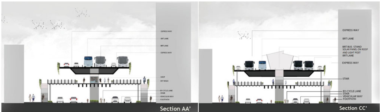
Fig. 10 Conceptual expressway with intermediate skywalk connected to the adjacent buildings. The existing road at ground level works a local road and cycle lane. Median and sidewalks are lined by plantation
