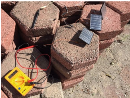
Fig. 3 Photoelectric cells connected in series
