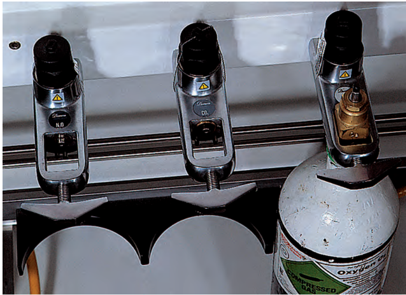
Fig. 1.5 Anaesthetic machine cylinder yokes. For the sake of comparison, the Bodok seal is absent from the nitrous oxide yoke (left).
