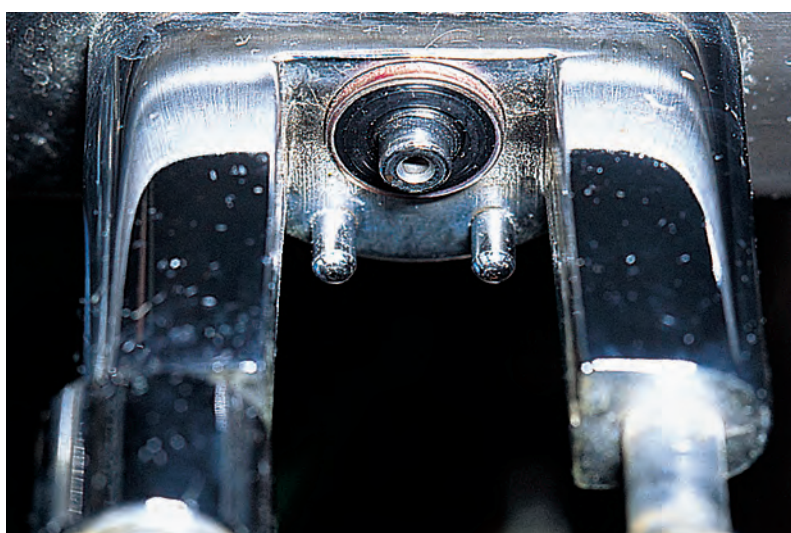
Fig. 1.8 A cylinder yoke and pin index system. Note that a Bodok seal is in position.
