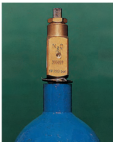
Fig. 1.6 Chemical formula ( N_2O ) engraved on a nitrous oxide cylinder valve.
