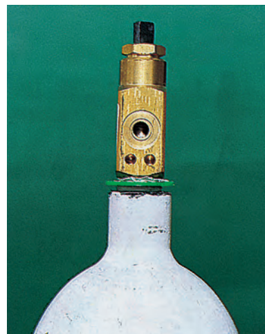
Fig. 1.2 Oxygen cylinder valve and pin index.
