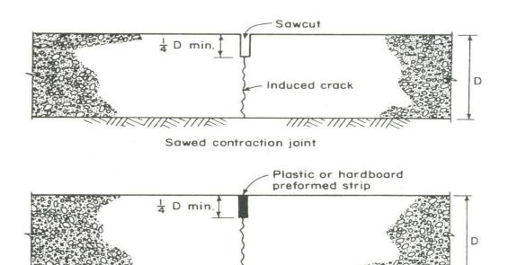
Premolded insert contraction joint
