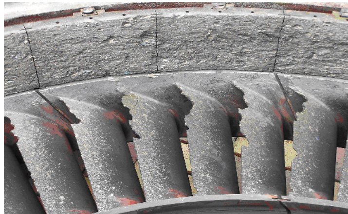
Gas Turbine Damage from FOD
