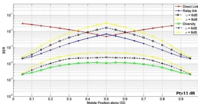
**Figure 4:** The effect of distance dependent path loss and Log-normal shadowing on BS cooperation systems.
