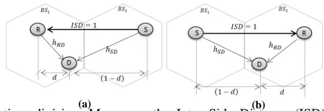
time division. Moreover, the Inter Side Distance (ISD) between the two BSs is normalized to one, and the MS moves on a straight line along the ISD. In addition, a high speed loss-less link is available between relay-destination for uplink mode and source-relay in downlink mode as shown in Fig. 1 and Fig. 2.
