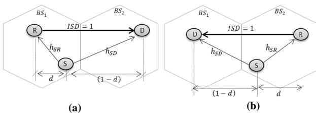
**Figure 1:** Uplink system Model. (a) MS served by BS<sub>1</sub>.
