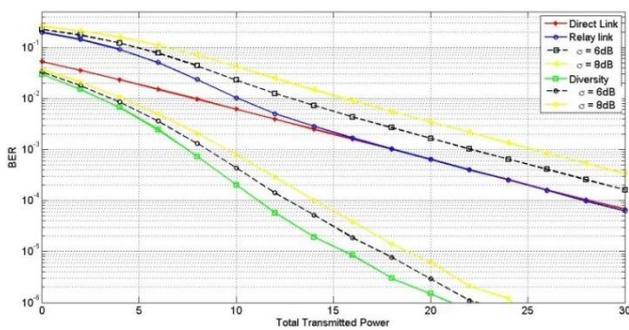
**Figure 3:** BS cooperation performance mode with Log-normal shadowing effect.
