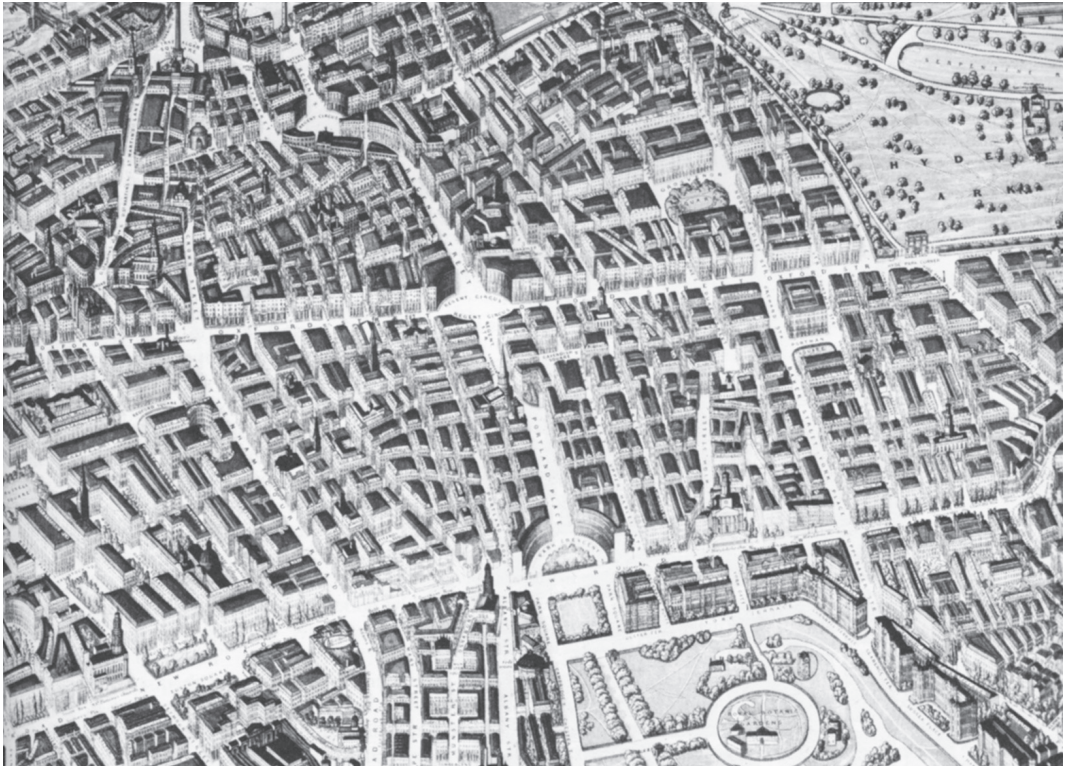
The emergence of the supergrid in the fabric of 19th Century London. These 'urban high-ways' of the 19th century are 'grounded' along their lengths by their immersion in a finer, slower, local grid.
