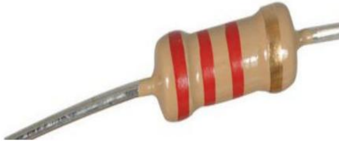
Figure 2.5 : 2.2k ohm and 0.25-watt capability, color code Red-Red-Red
