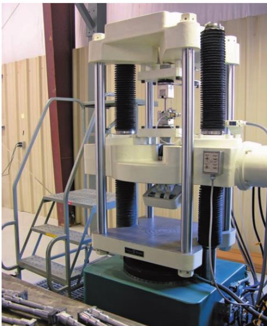
Figure 11- This machine is used to test tensile-test specimens
