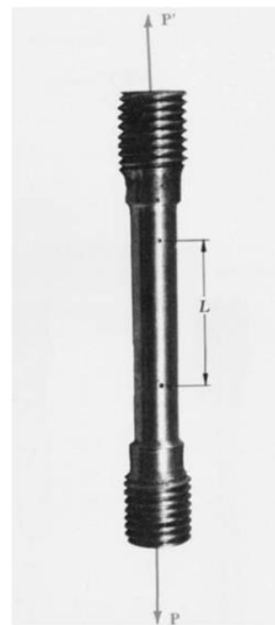
Figure 10- Test specimen with tensile load
