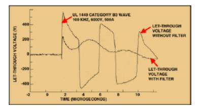
Filtering is often referred to as "sine wave tracking" or "active tracking." These are marketing terms, and are not relevant to filter performance. Also, not all SPDs provide filtering. Many SPDs claim to possess sine wave tracking, sine wave contour, or EMI/RFI noise attenuation, but may not employ a quality filter.
