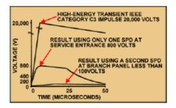
In the case of a residential application, the second-stage protection can take the form of a surge strip. That is, provided it offers protection for all of a load's exposures:
