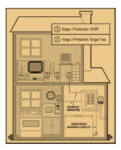
Let's also consider an industrial application. The first stage of protection is provided at the service entrance, with an SPD integrated into the *Switchboard* or main *Panelboard*. The second-stage protection can take the form of a critical load protector (such as a filtering device), or an SPD at the power panel that feeds critical loads.
