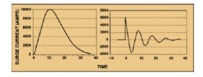
The combination wave waveform is a unipolar pulse, similar to a lightning strike.
