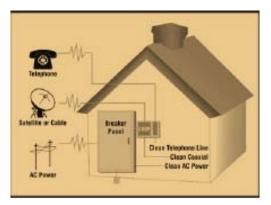
For this reason, surge protective devices (SPDs) should be installed at the service entrance on all metal conductors.
