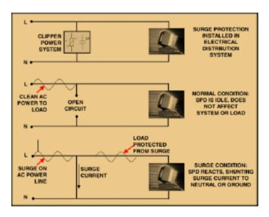
Figure 17. The MOV Protects Equipment from Harmful Surges
