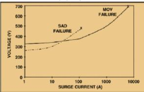
Figure 14. The SAD has Less Energy Capability, Shorter Lifespan than the MOV
