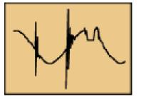
A surge can travel on any metallic conductor entering a building. Electrical, telephone and coaxial cable lines make great surge conductors.
