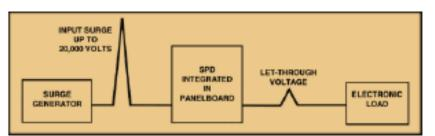
Figure  $\mathbf{Y}$ . Example of SPD Integrated in a Panelboard
