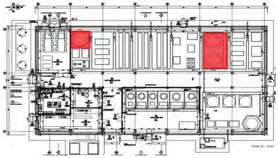
Roof bracings and purlins between axes WC-WH/1-2 should be erected after the erection of interior platforms. In case of any changes in the equipment locations, the Owner will be informed about these situations and works will be progressed accordingly.
