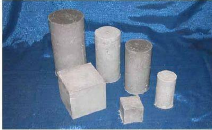
Figure(5): Cube and Cylinder Specimens for Compression Strength Testing.
