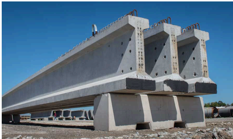
Fig. ١٤ precast concrete girders
