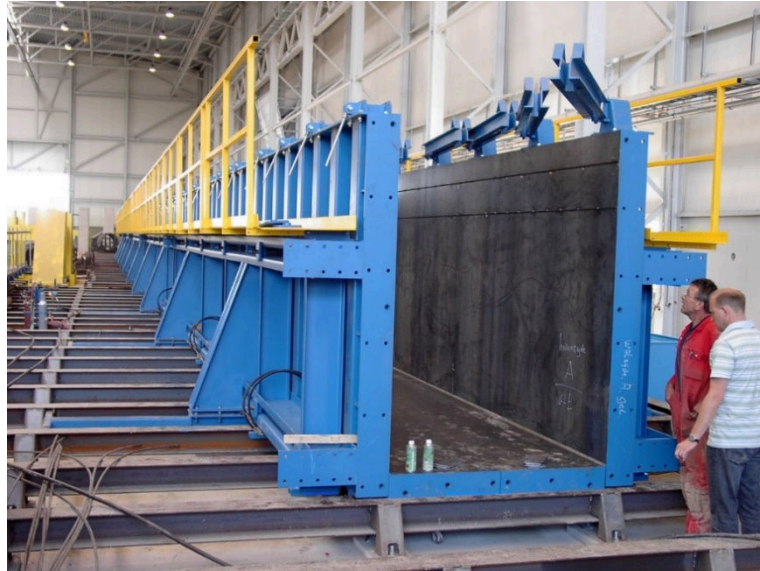
Fig. 1 Steel mould made by Hendriks Precon Co. (Netherlands)
