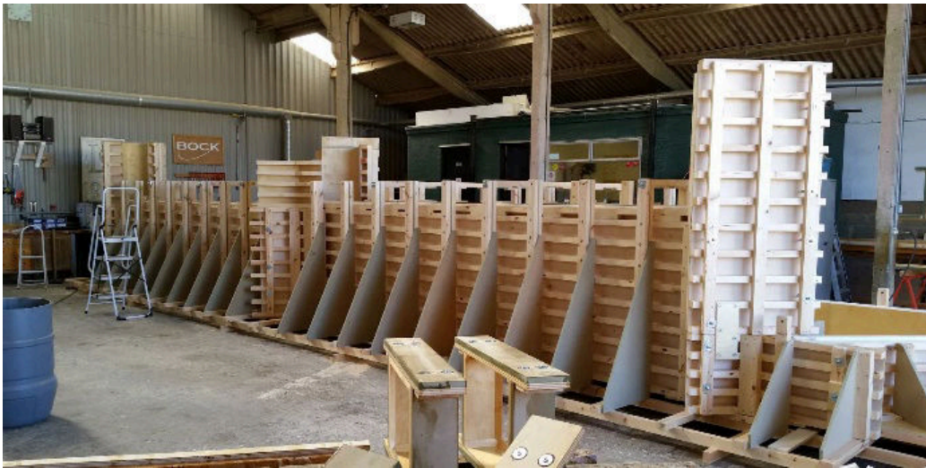
Fig. 1 Wooden mould made by Invictamoulds Co. (England)
