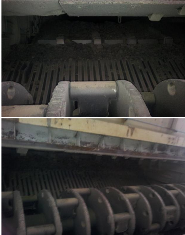
Figure 5 Internal of Claudius Peter Cooler with Crusher of clinker
