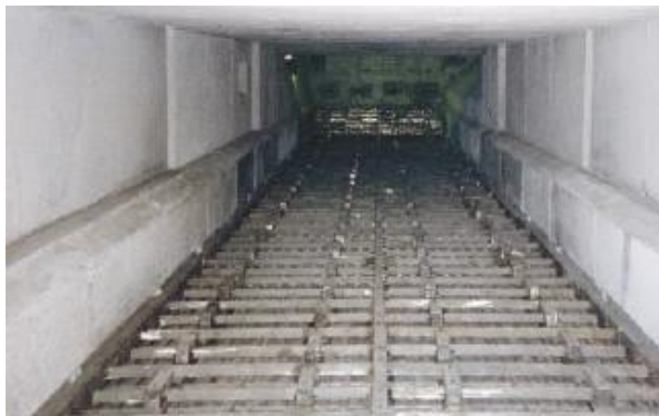
Figure 6 Internal of Claudius Peter Cooler with Crusher of clinker
