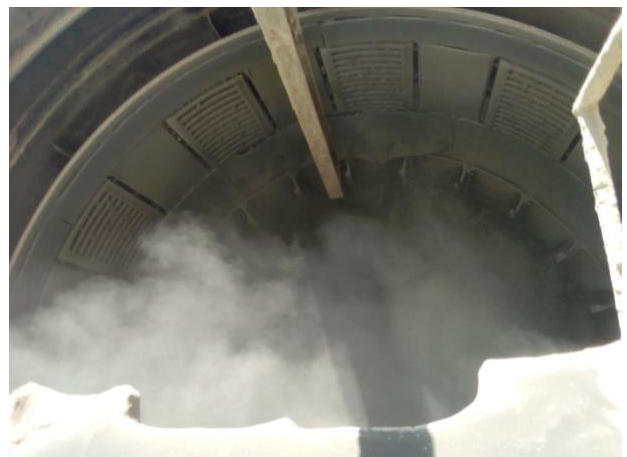
Figure 7 Rotary type cooler and internal view of it
