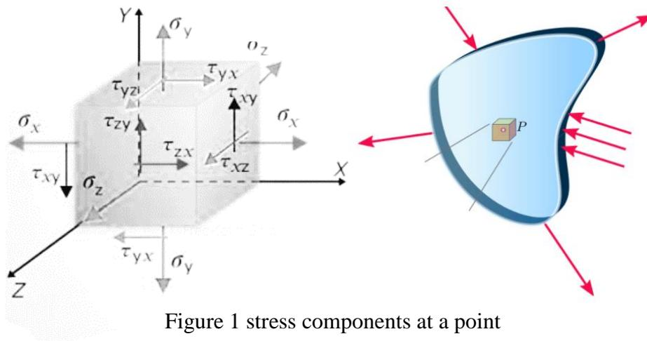
Figure 1 stress components at a point
