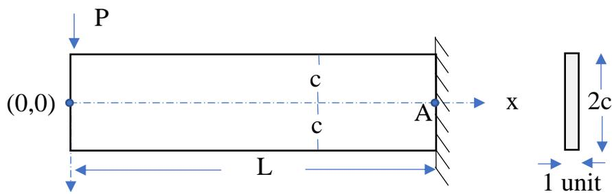
Figure 4 cantilever beam narrow rectangular cross section
