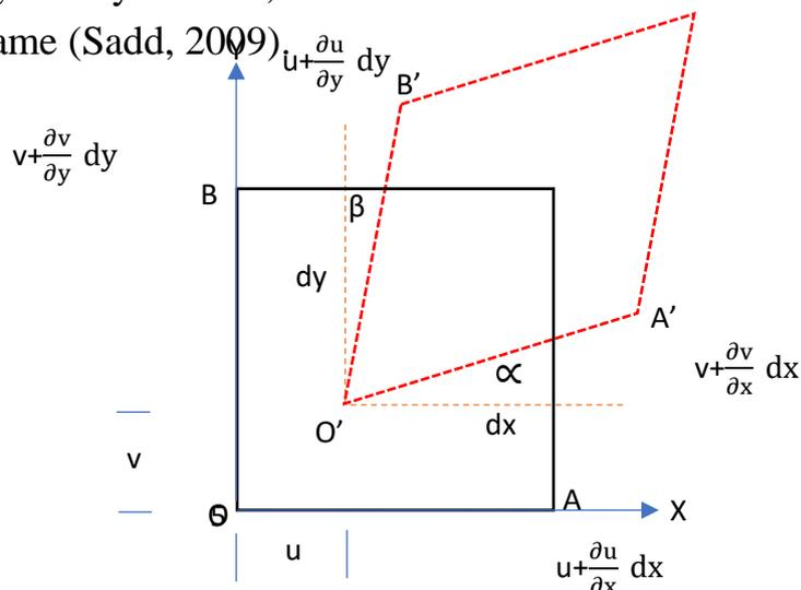
Figure 2 Two-dimensional geometric strain deformation.
