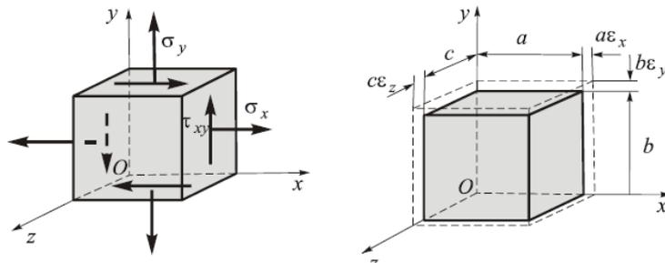
Figure 3 Element of material in plane stress and normal strains
