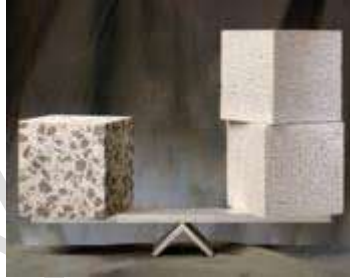
HySSIL is as strong as normal concrete but only half as heavy
