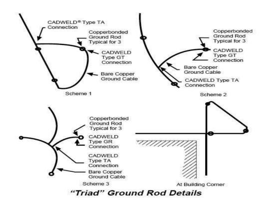
Triad arrangements are not recommended unless the spacing between the ground rods is equal to or greater than the individual ground rod length.
