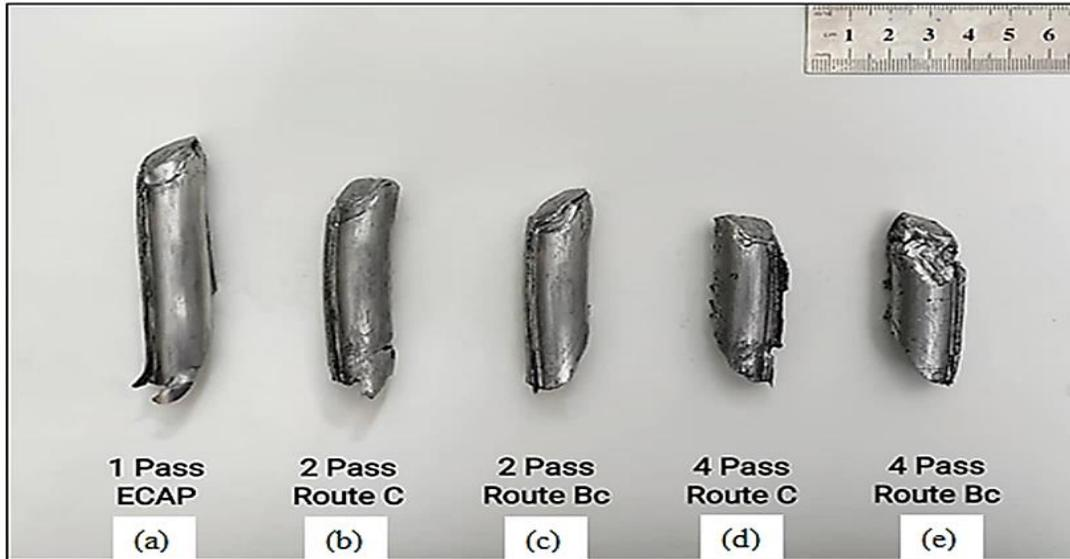
Figure 5: Final products of solid-state recycling of AA6061-T4 alloy recycled chips.
