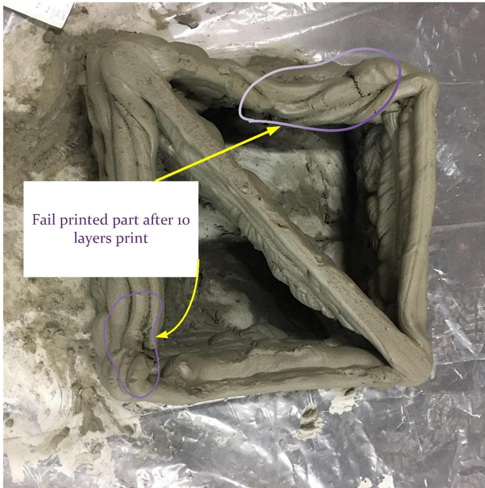
Figure (11) The movement of the robot arm has a major effect on the printing process, particularly when the height of the object increased to more than 7 layers.
