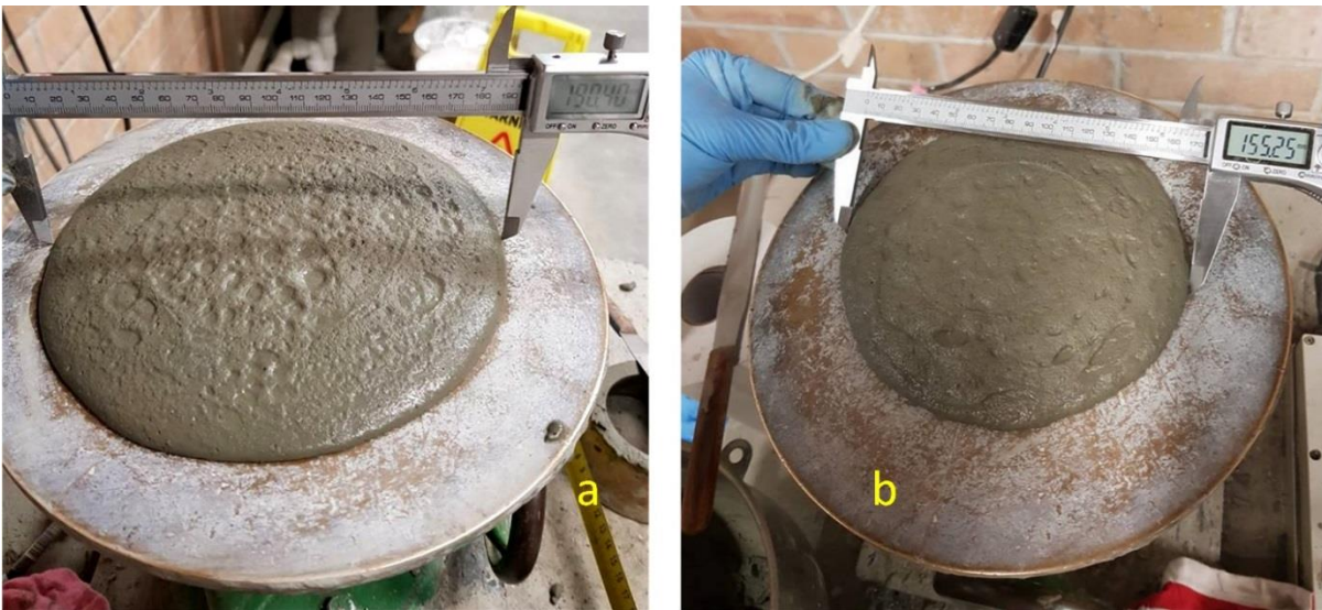
Figure (16) Spread-flow test: (a) for trial 5 which did not use fibre; (b) for the same trial by adding fibre with 1% polypropylene fibre.
