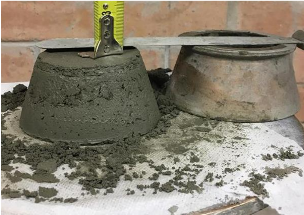
Figure (15) Mini-cone slump test for trial 8.
