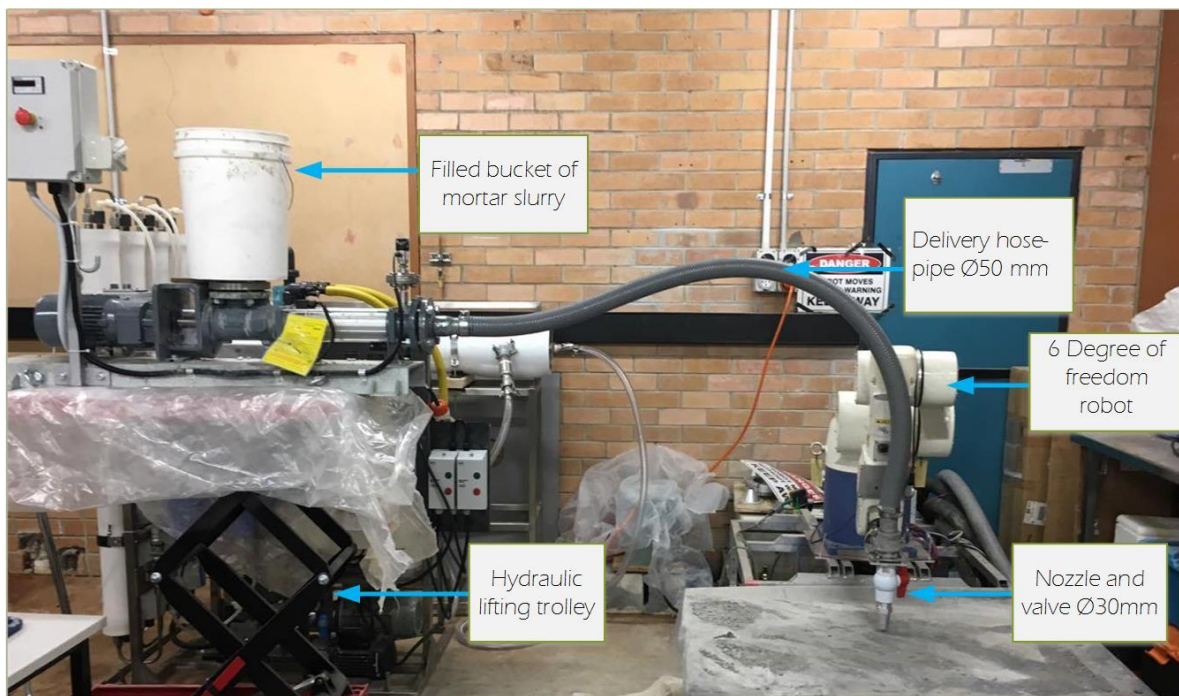
Figure (4) The final system with the progress cavity pump connected to the robot.
