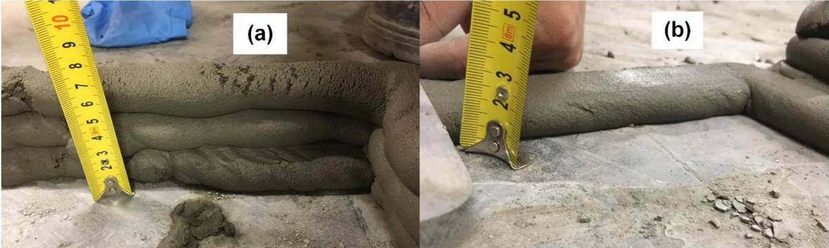
Figure (10) (a) Three layers of the printed object; (b) One layer of the printed object.
