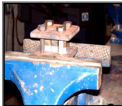
Figure 1: Fixture and assemblies for diffusion welding specimens
