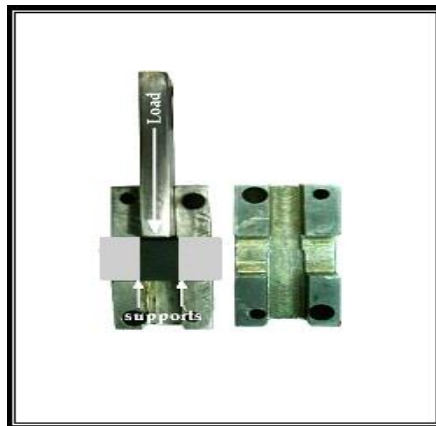
Figure 3: Punch and die used in shear test
