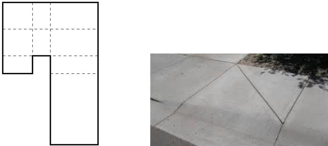
Figure (5): Correctly laid out joints.
