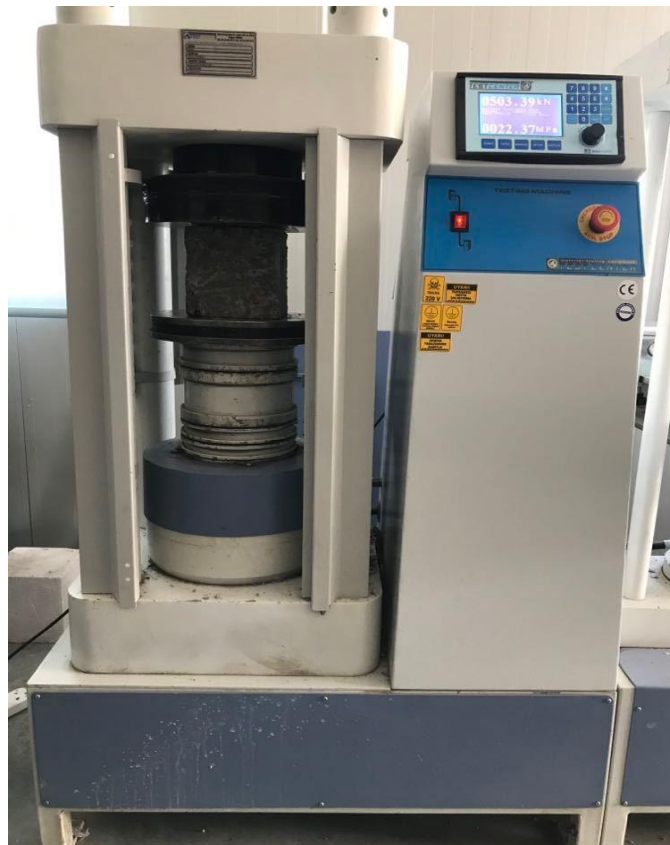
Figure 3-10: Compressive Strength Machine.
