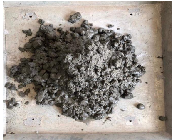
Figure 4-8: Slump Test at (C2).
