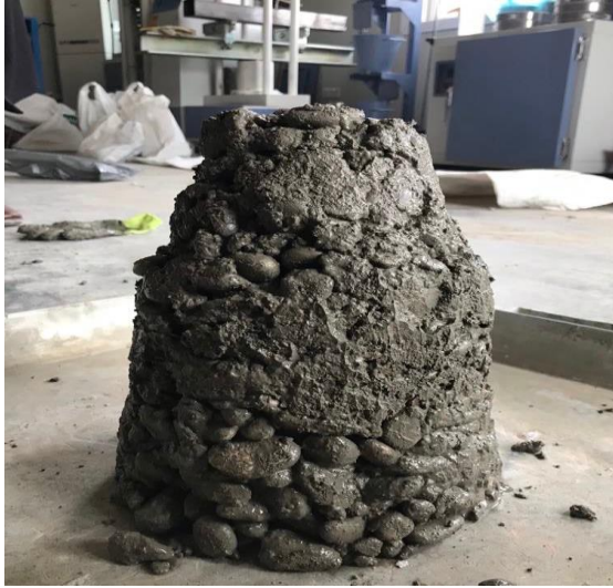
Figure 4-7: Slump Test at (C1).
