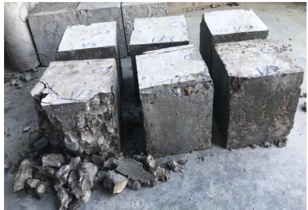
Figure 4-16: The Compressive Specimens (C3).
