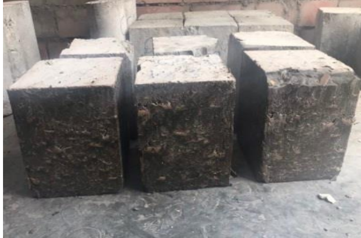
Figure 4-18: The Compressive Specimens (C5).
