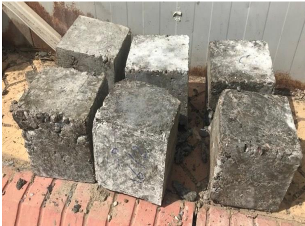
Figure 4-13: The Compressive Specimens (C0).
