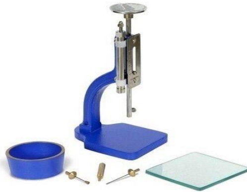
Figure 3-7: Initial and Final Setting Time of Cement with Vicat's Apparatus.
