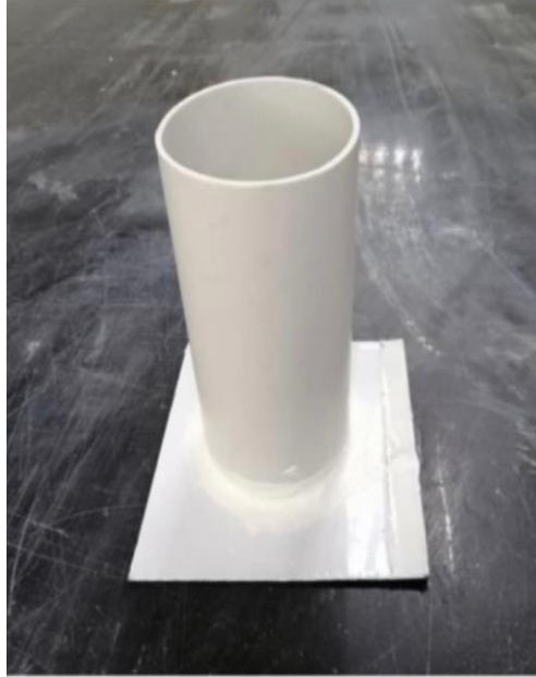
Figure 3-11: Standard Cylinder of 100 mm x 200mm.
