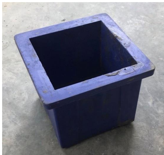
Figure 3-9: Standard Cube of 150mm x 150mm x 150 mm.
