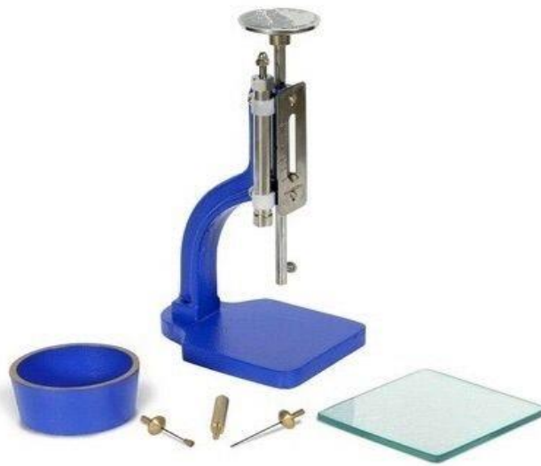
Figure 3-6: Normal Consistency of Cement with Vicat's Apparatus.
