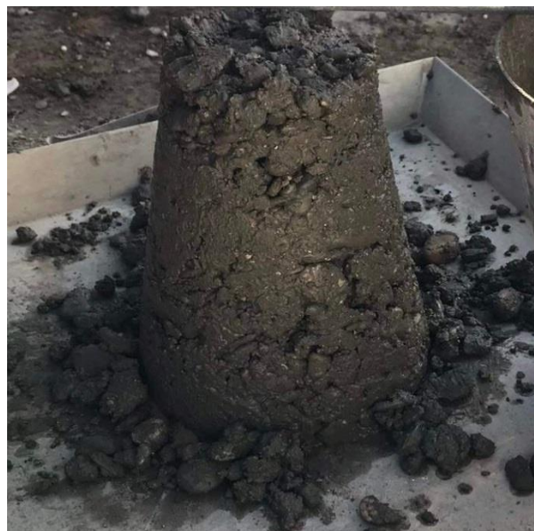
Figure 4-6: Slump Test at (C0)
