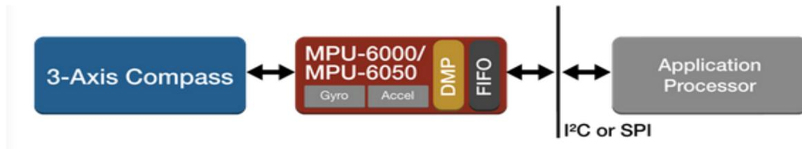
Figure 3.4: MPU6000 system diagram (after InvenSense webpage)
