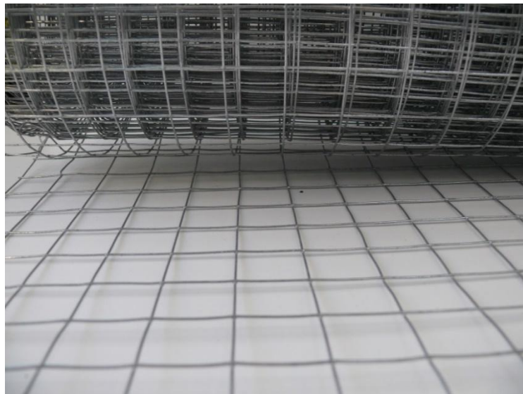
Fig. 3. 1 Galvanized square welded wire mesh with opening of ( 19× 19 ) mm and an actual strand diameter of 1.90mm
