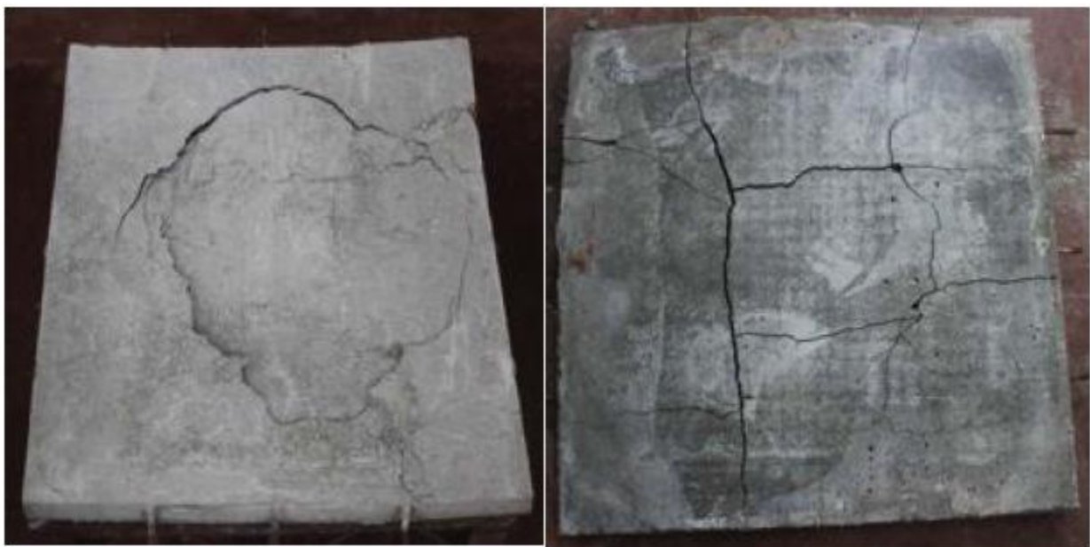
Fig. 3.9 The Crack Patterns of the Top (Left) and Bottom (Right) of the Prototypes
