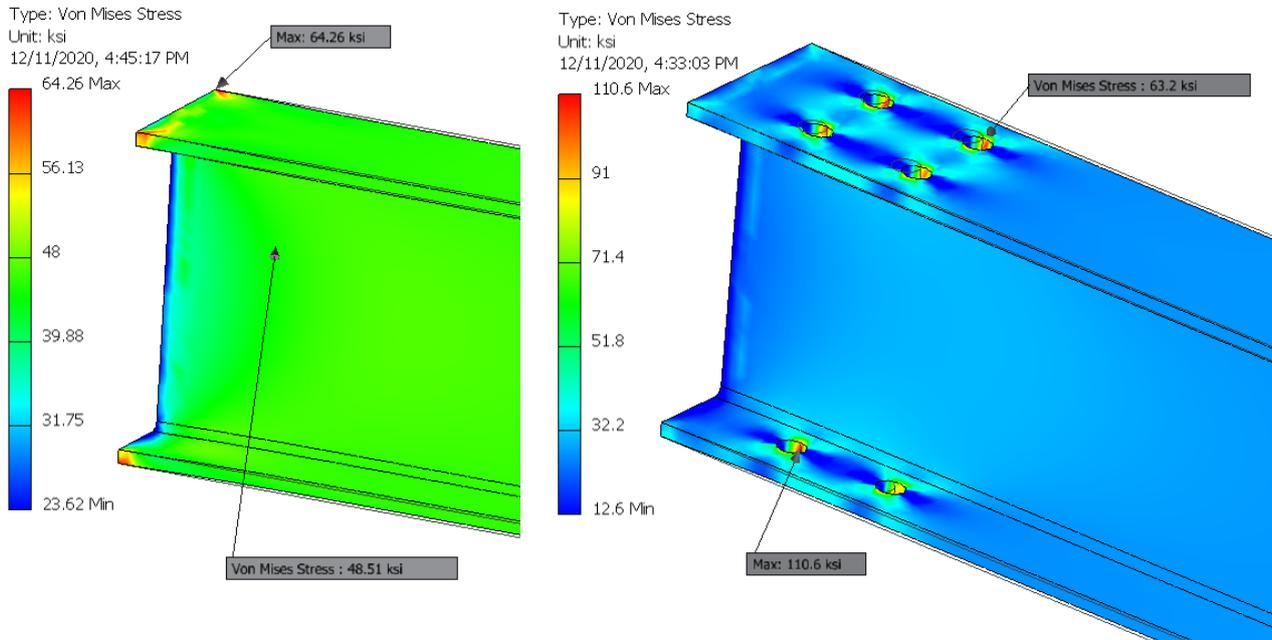
Figure 7 Sample two EFM stress **is resulted** by Autodesk Inventor **with** holes and without hole
