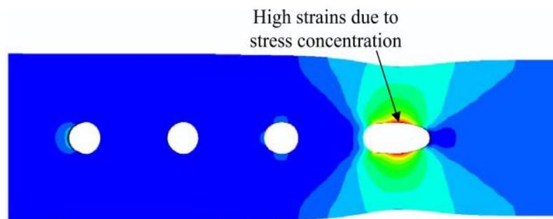
Figure 1 Typical FE model failing in net rupture from the parametric studies (Lutfi and Salih, 2010)
