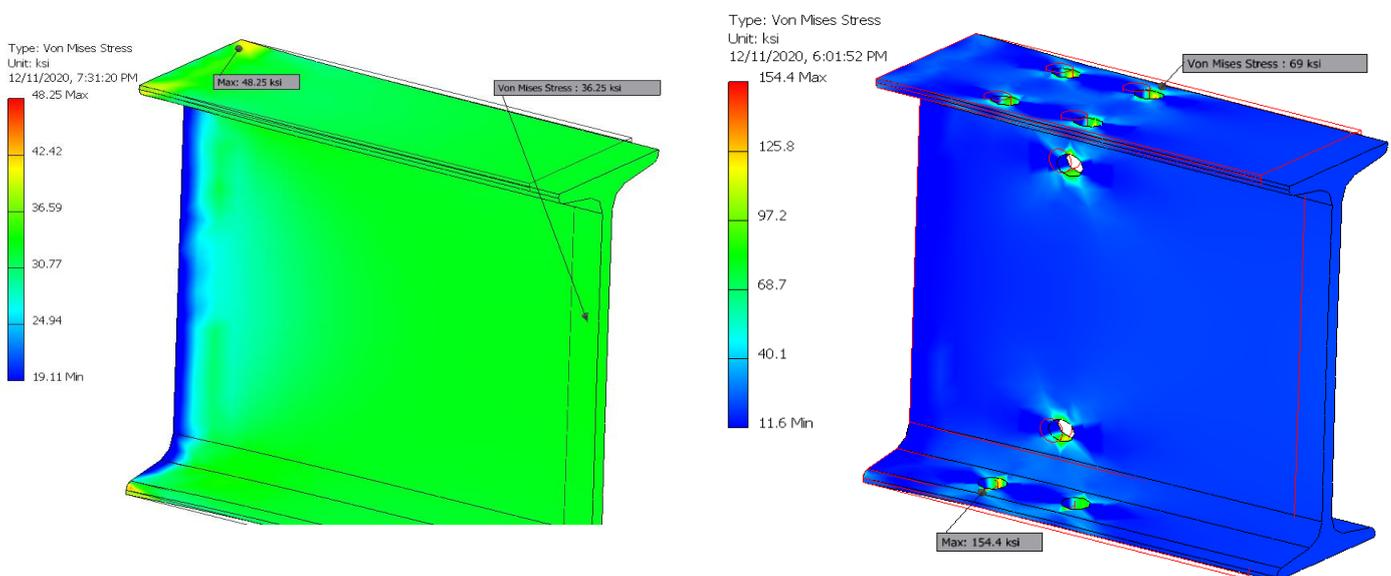
Figure 8 sample three EFM stress is resulted by Autodesk Inventor with holes and without holes
