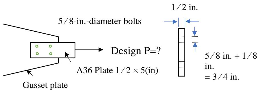
Figure 5 steel plate (Segui, 2012)
