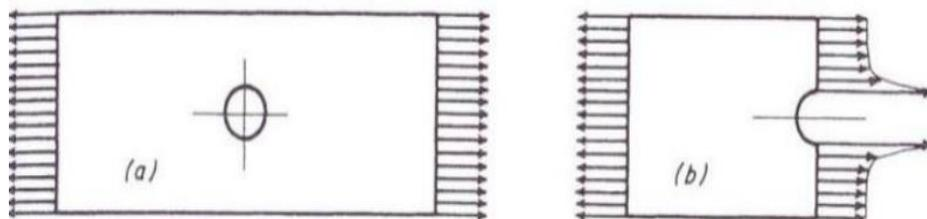
Figure 2 Stress distribution for a plate subjected to tensile load (a) away from the hole; (b) the section of the central hole (Spotts and Shoup, 1999).
