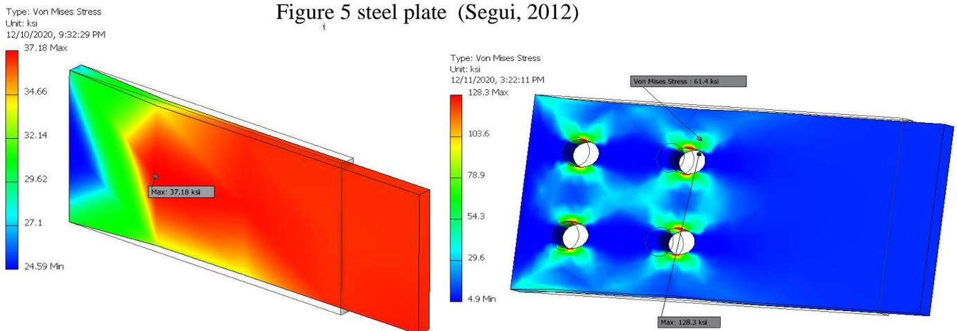
Figure 6 Sample **one** EFM stress **is resulted** by Autodesk Inventor with holes and without hole.
