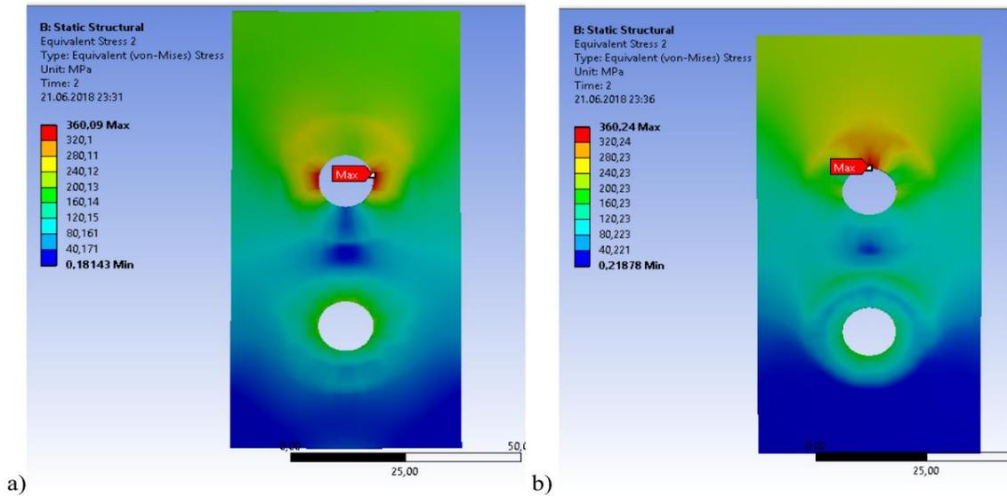
Figure 4 Diagram of bolted connection stresses: a – in tension element, b – in compression elements. (Ustimenko and Skachkov, 2020)
