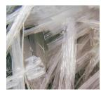
Polypropylene fiber which is classified as number °-PP (plastic polymer). Transformed from propylene, it has similar properties as polyethylene but it is harder and more heat resistant, used in a variety of applications.
