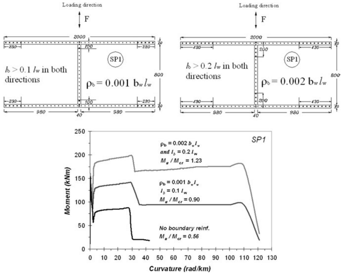
Figure 10. Comparison of moment–curvature diagrams for section with and without boundary reinforcements for loading along weak axis (SP1)
