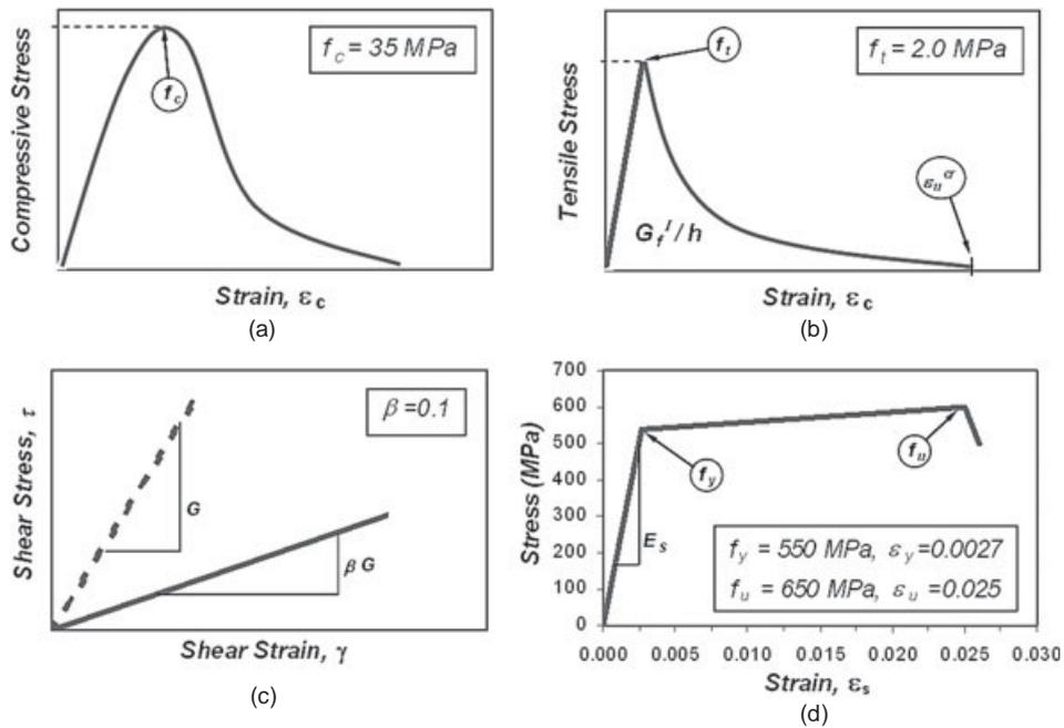
Figure 3. Concrete and steel nonlinear material models: (a) unconfined concrete model; (b) nonlinear tension-softening model; (c) shear retention; (d) reinforcement steel model
