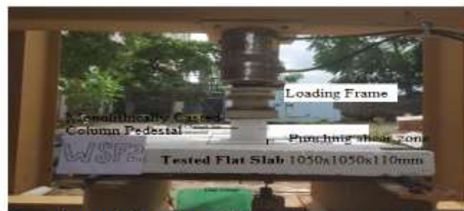
Experimental Testing of Flat slabs (NSF, WSF1, WSF2) Fig.8
