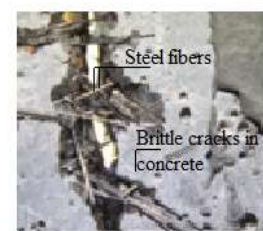
Fig.3. Shear Resistance of Steel fibres
