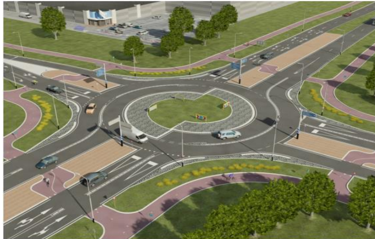
Figure 7: (Fortuijn turbo roundabout, Netherland)
