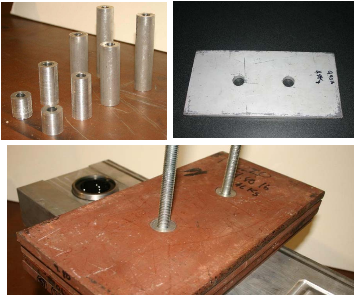
Figure 3-8: Machined Aluminum spacers (left) mass plates with pre-existing holes (right) and spacers placed inside the weights (bottom).
