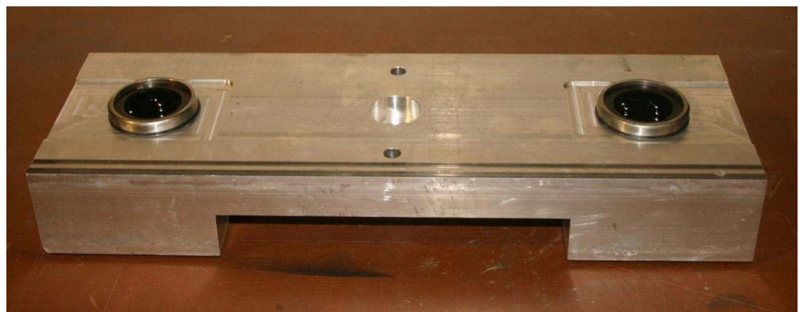
Figure 3-7: CAD Drawing of brace (top) and machined brace with bearings insert (bottom).
