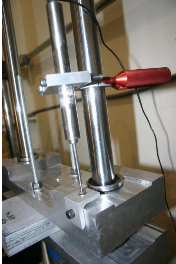
Figure 3-10: LVDT mounted to upper brace using custom machined bracket.
