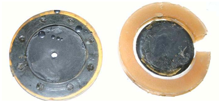
Figure 3-12: Metal-elastic mount that failed under high amplitude testing.
