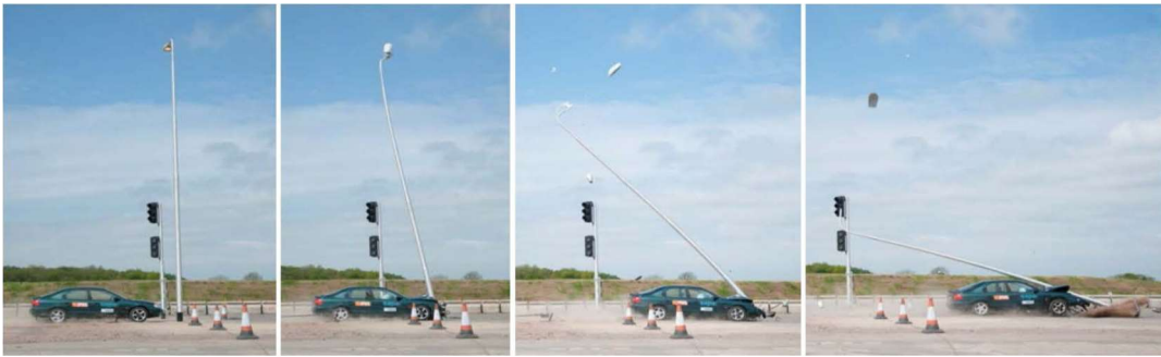
Figure 17: Breakaway devices (Passive Safety Pole)
