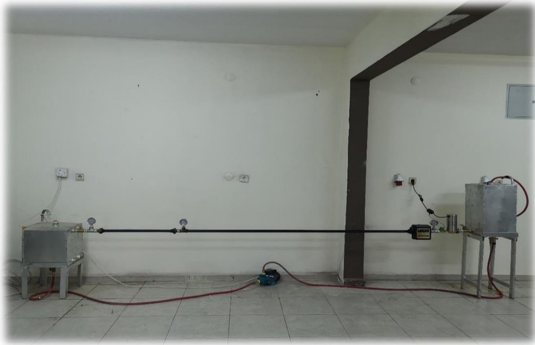
Figure(4) Experiment setup the carbon steel pipe which was appropriate for transporting crude oil has been used in conducting the experiment.
