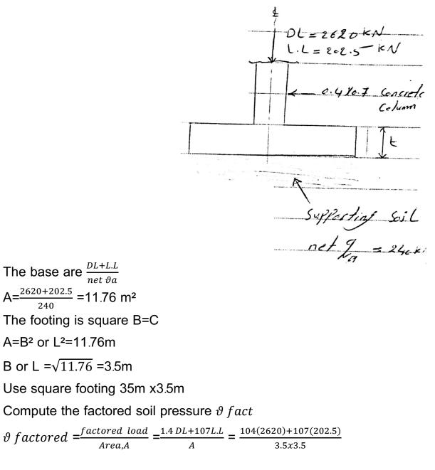
=  $32.8 \ knlm^2$ Vc =  $\frac{0.85}{6} = \sqrt{21} = 0.65 \ *1000 = 650 \text{knlm}^2$ The applied shear force = B<sup>2</sup>  $\vartheta fact = (3.5)^2 \text{x} \ 328$ =4018 kn
