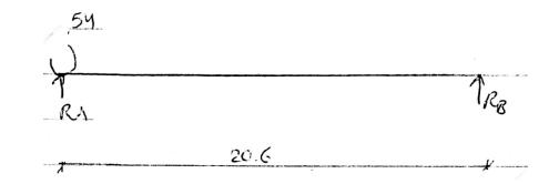
Rmax=101.25kn Pu(external)= Wd.L +WL.L =2620+ 202.5 =2822 kn Pu external= 2822 <3358 kn 0.k
