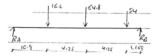
$\sum MA = 0$ -RBx20.6+16.2x10.9+64.8x15.15+54x19.4 RB=107 kn VL.L = 0.9x107 =96.4 kn VI=0.26x 107=27.8 kn Vu=27.8+9604+228=352 kn
