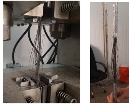
Figure 5. Aluminum anchors Figure 6. Tensile test of BFRP bar with aluminum anchor
