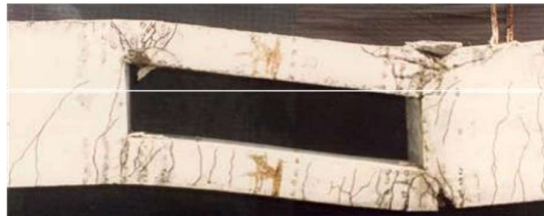
Figure 5.17 A suitable reinforcement scheme for the large opening.
