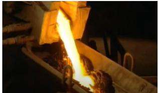
3. Fiberization: Spin the molten material into fine fibers using high-speed spinning equipment.
