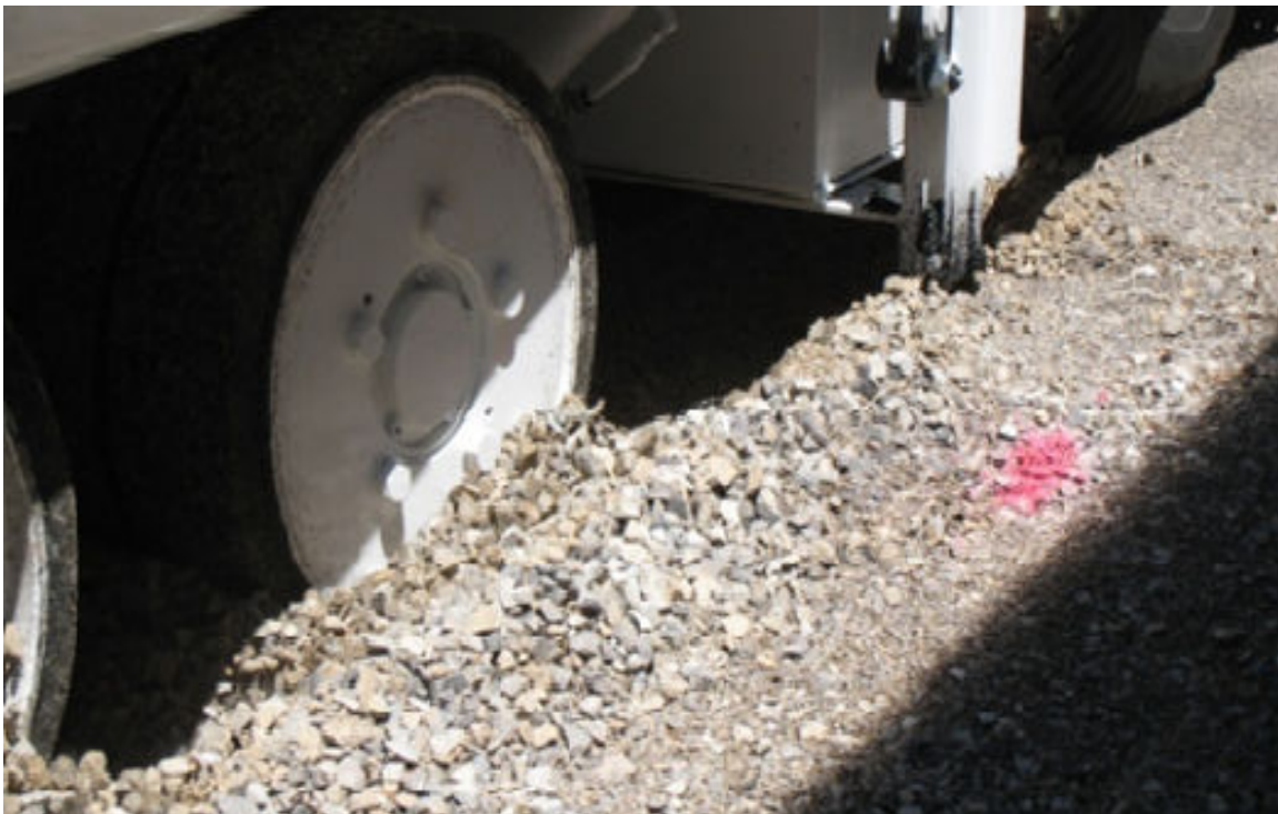
Figure 2-9-11. Yielding Granular Base
