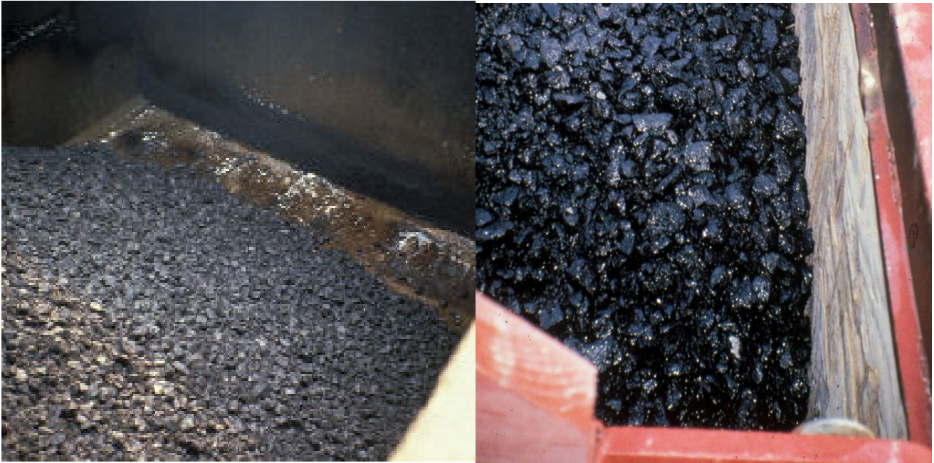
(Figure ١- ٤) End of Truck Segregation
