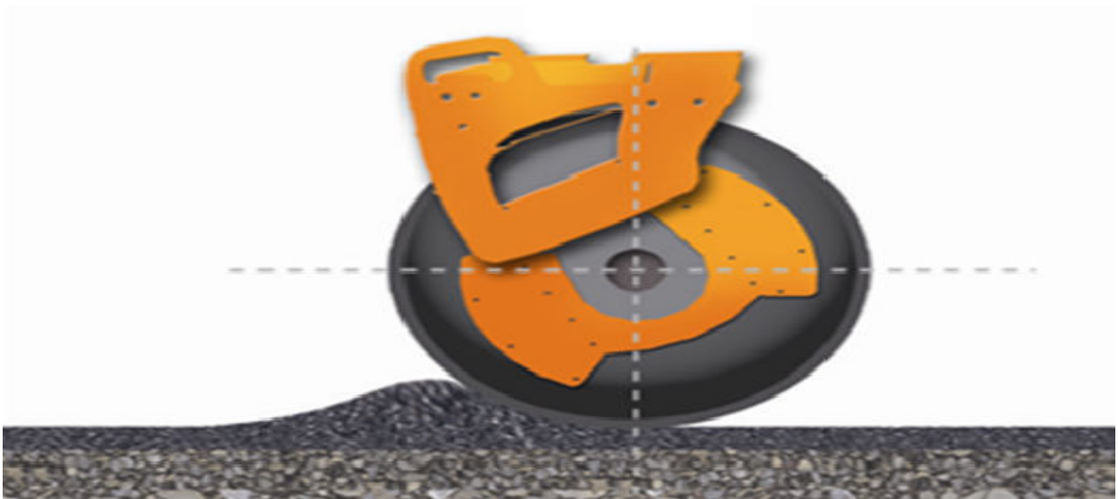
Figure ∩-∩. Mat Shoving Ahead of Roller
