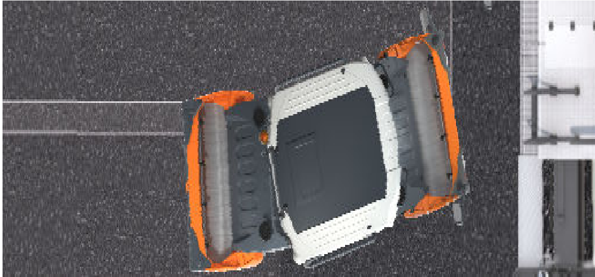
Figure 3-3-2. Stopping Roller at an Angle
