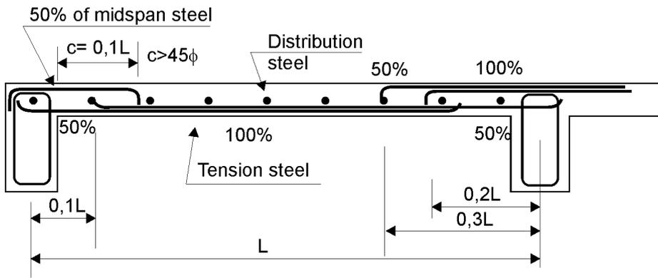
**Curtailment of steel in beam and slab construction.**
