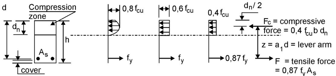
A partial material factor of 1,15 is applied to the steel and 1,5 to the concrete.
