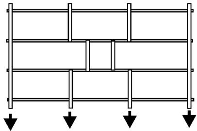
Structurally undesirable uncomfortable diversion of main loads sideways.
