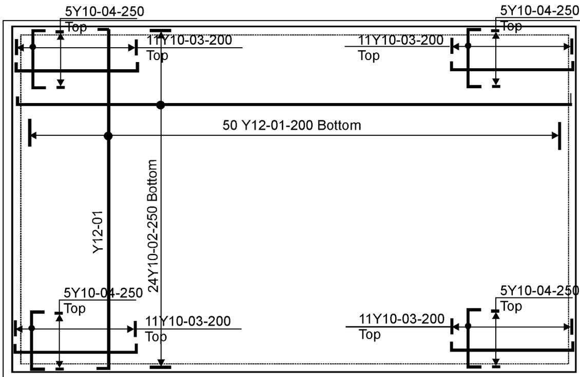
**Typical layout for a simply supported flat slab.**
