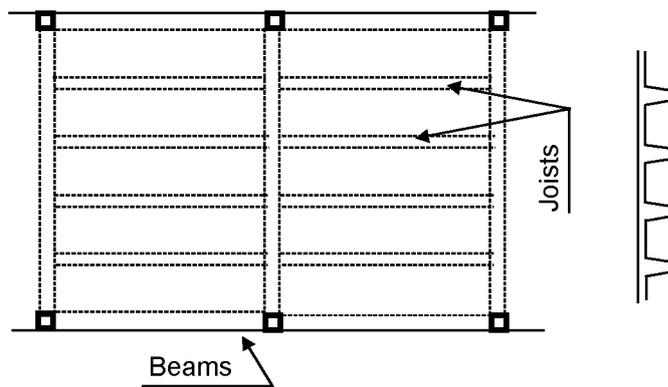
One-way joist and girder
