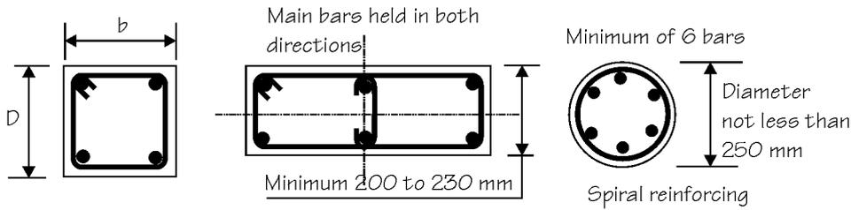
*b* not less than 225 mm especially where down pipes are placed in the columns.
