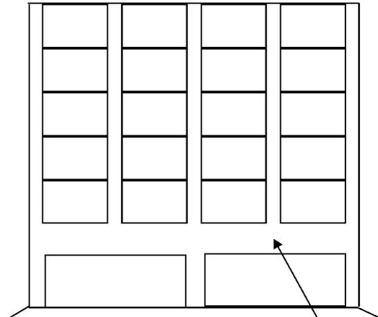
Deep beam picks up intermediate column loads from main grid above.
