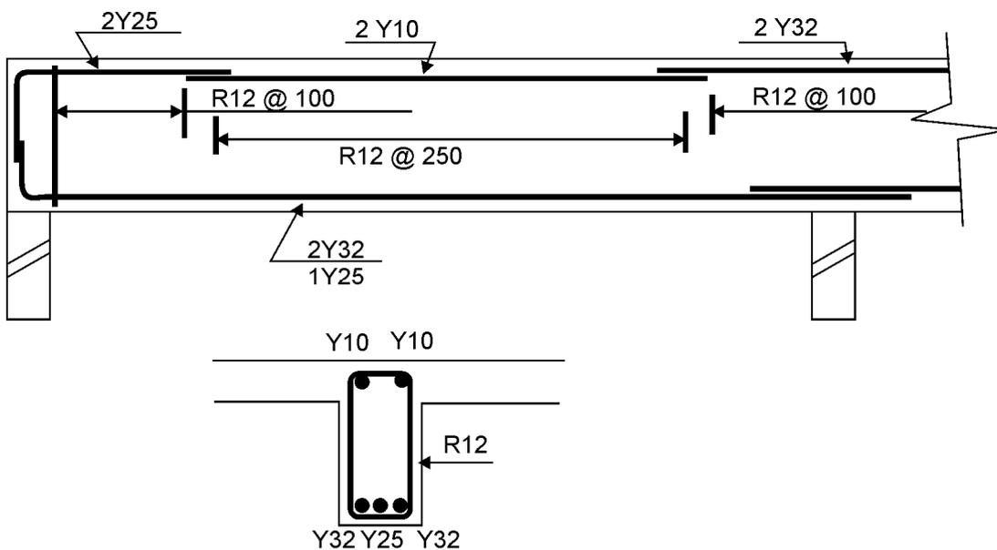
**Typical steel detail for concrete beam.**
