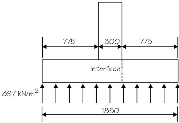
$$M_u = (397 \times 1,85) \times 0,775 \times \frac{0,775}{2} = 220,6 \text{ kN.m}$$
