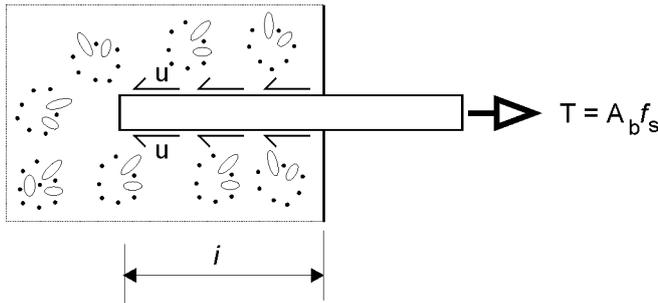
The bar has a cross-sectional area  $A_b$  and a stress of  $f_s$  is developed. This must be in equilibrium with the forces induced in the bond. The bond stresses are  $= u$  and the shear area is the circumference times the bond length  $l$ . One would like to ensure that the bond does not break before the steel bar yields. If the maximum bond stress is  $u_{max}$ , then:
