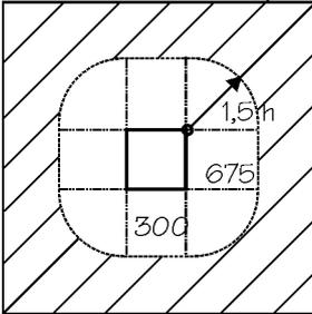
$$\begin{aligned} \text{Punching circumference} &= 4 \times 300 + \pi \times D \\ &= 4 \times 300 + \pi \times 3 \text{ h} \\ &= 4 \times 300 + \pi \times 3 \times 450 \\ &= 5441 \text{ mm} \end{aligned}$$
