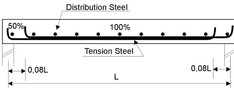
**Curtailment of tension steel in simply supported slab construction.**
