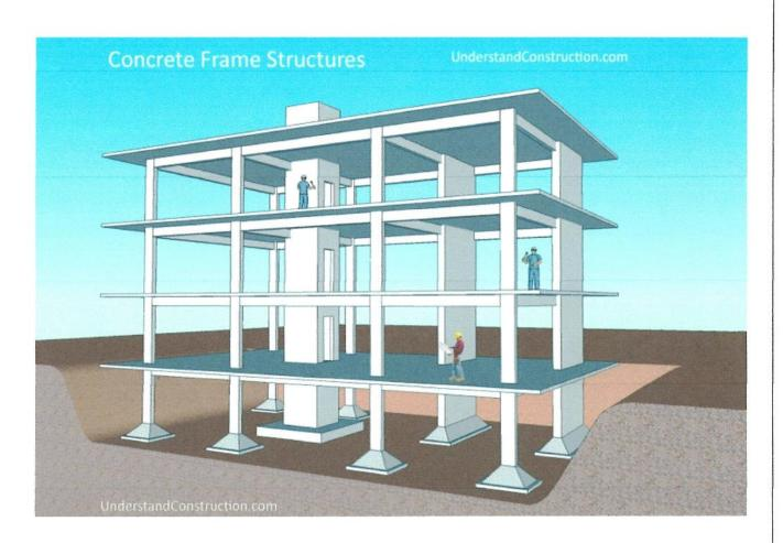
When we say concrete in the building trade, we actually mean reinforced concrete. Its full name is reinforced cement concrete, or RCC. RCC is concrete that contains steel bars, called reinforcement bars, or rebars. This combination works very well, as concrete is very strong in compression, easy to produce at site, and inexpensive, and steel is very very strong in tension. To make reinforced concrete, one first makes a
