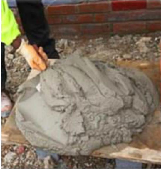
Figure 2 - (a) Conventional mortar Figure 3 -(b) Self-leveling mortar
