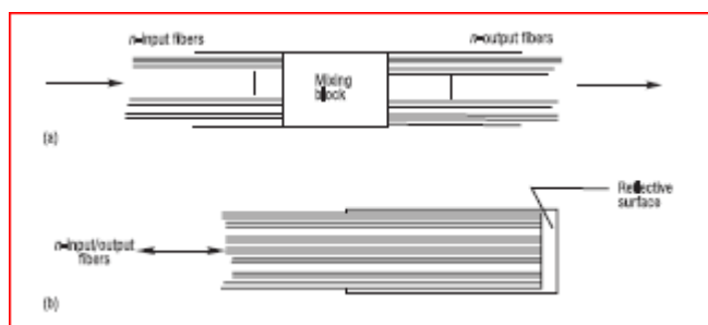
Figure 35 Star couplers (a) Transmissive (b) Reflective
