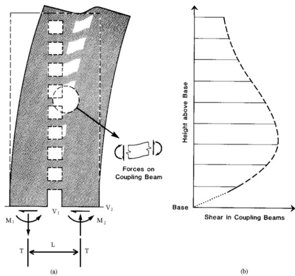
Figure 32. Laterally loaded coupled wall system. (a) Forces on walls at base. (b) Typical distribution of shears in coupling beams over height of structure.
