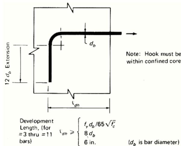
Figure 35. Development length for beam bars with  $90^\circ$  hooks.
