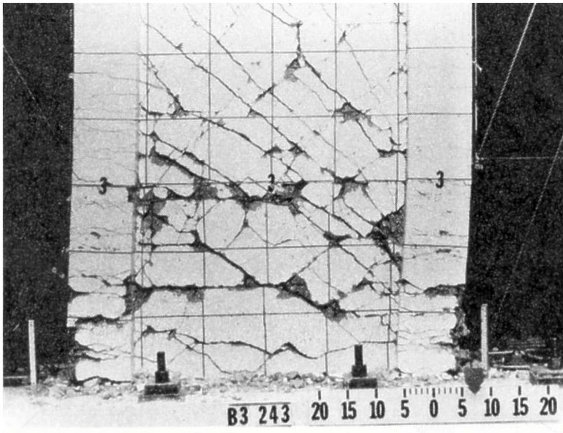
Figure 28. (a) Load-deflection curve of specimen subjected to load cycles of progressively increasing amplitude. (b) View of specimen at +8 in. top deflection. <sup>(53)</sup>
