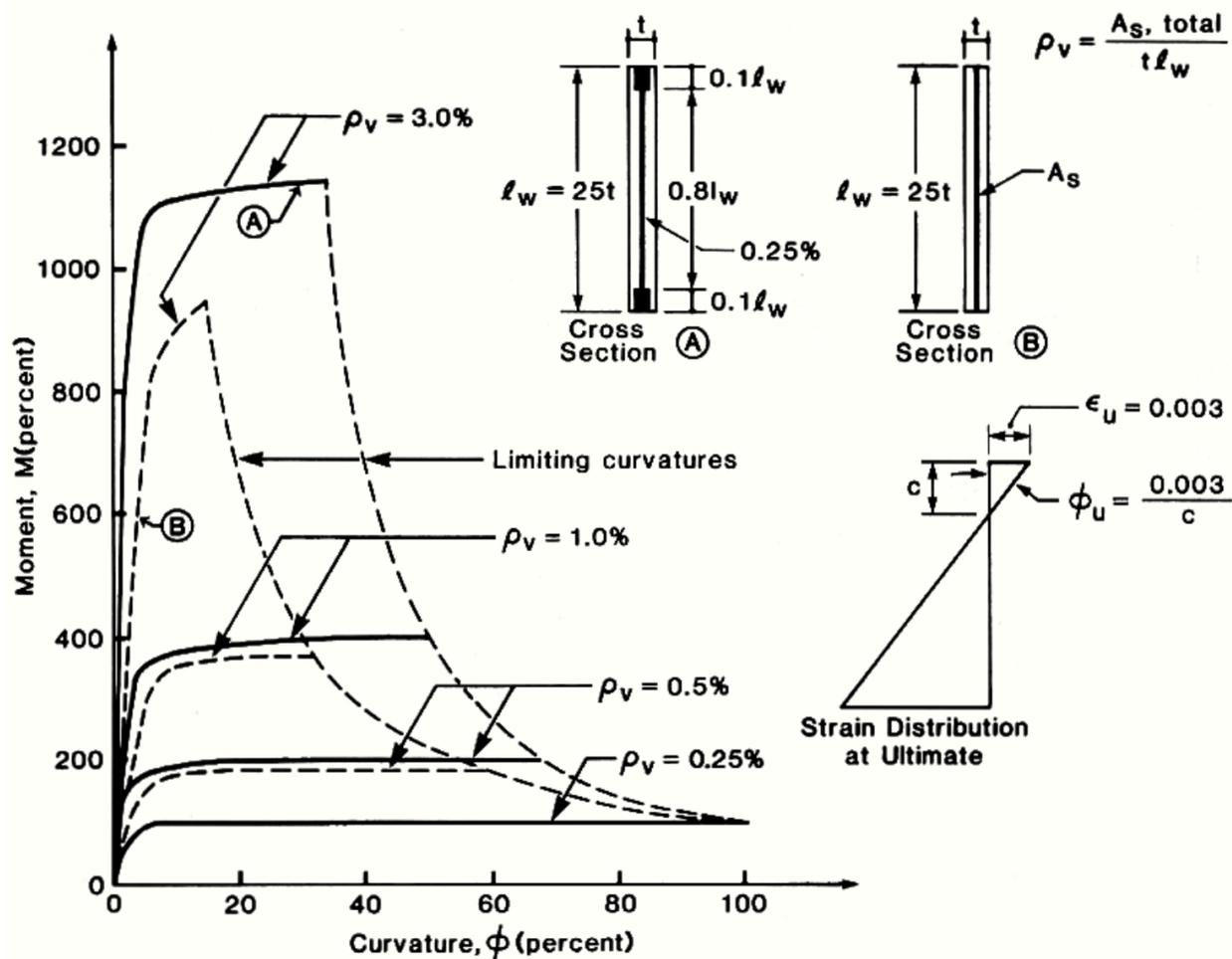
Figure 25. Moment-curvature curves for statically loaded rectangular walls as a function of reinforcement distribution. <sup>(52)</sup>
