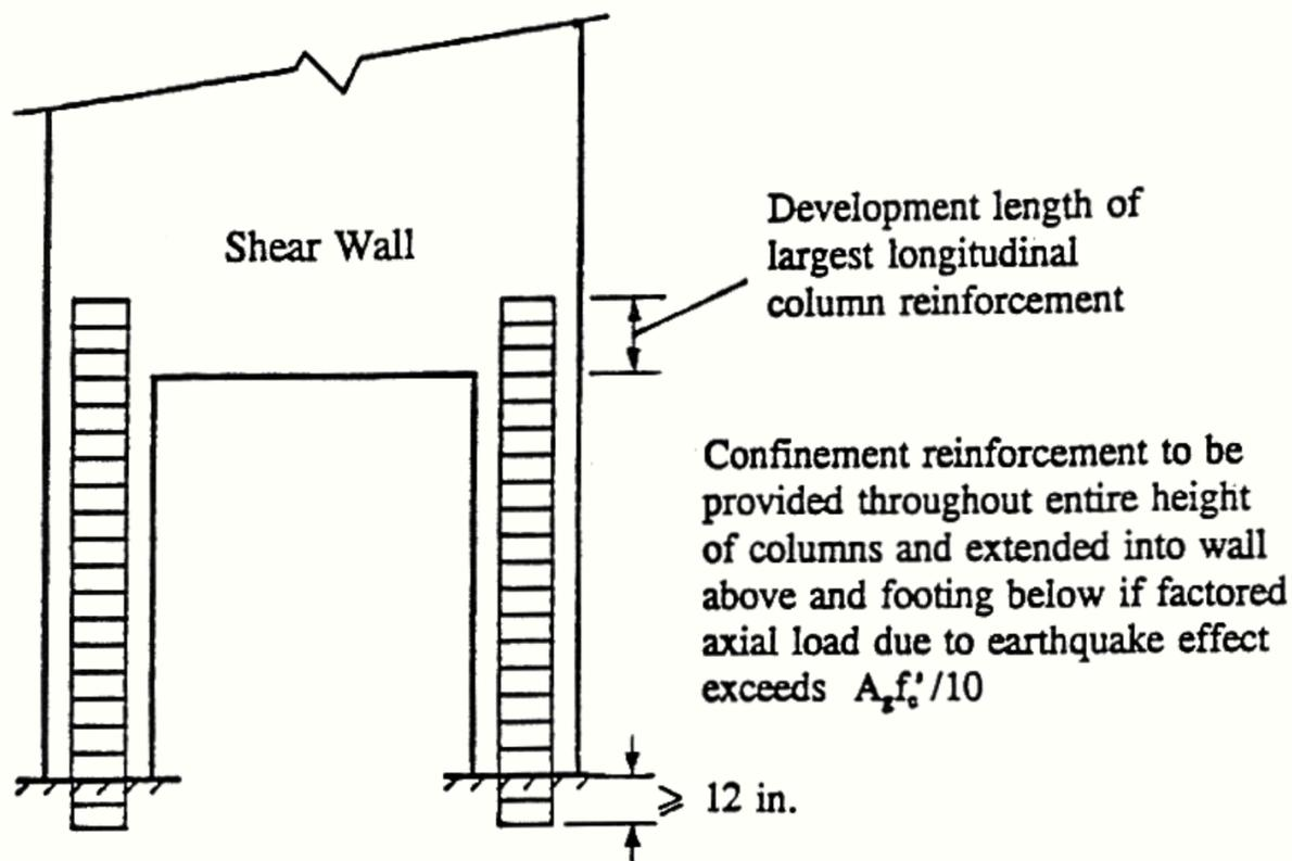
Figure 39. Columns supporting discontinued wall.
