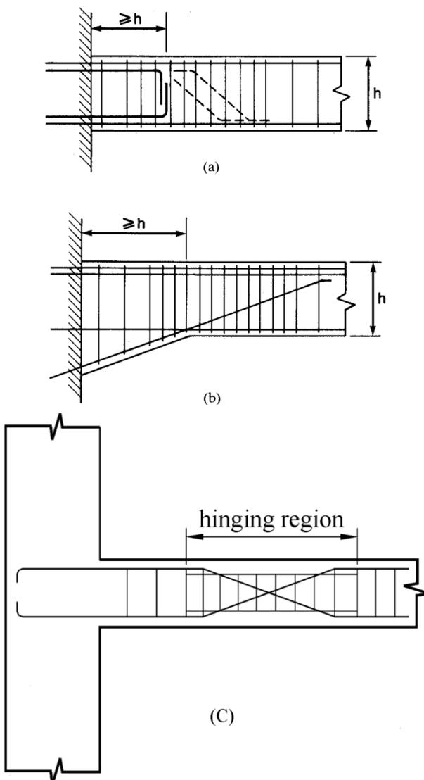
Figure 20. Proposed details for forcing beam hinging away from column face<sup>(26)</sup>. See also Fig. 15. (a) Supplementary flexural reinforcement. (b) Haunch. (c) Special reinforcement detail.
