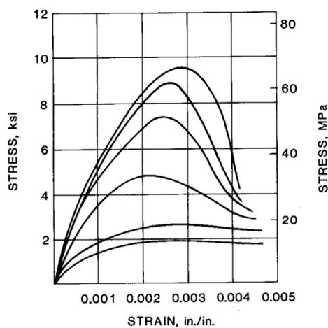
Figure 8. Typical stress-strain curves for concrete of varying compressive strengths.
