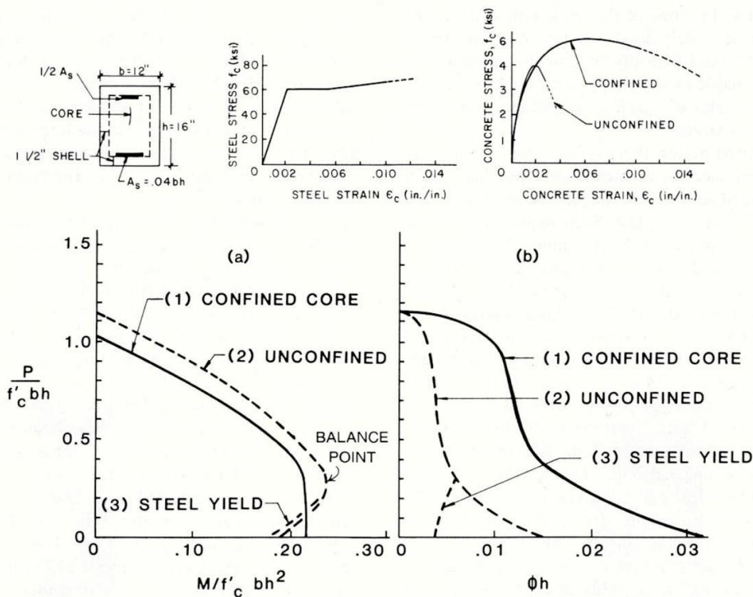
Figure 11. Axial load-moment interaction and load-curvature curves for a typical reinforced concrete section with unconfined and confined cores.
