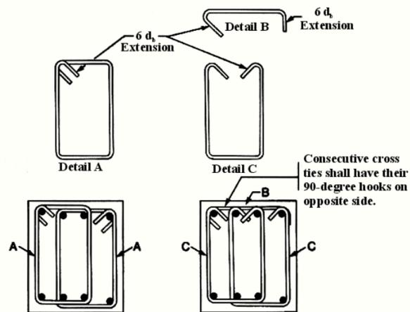
Figure 37. Single and two-piece hoops
