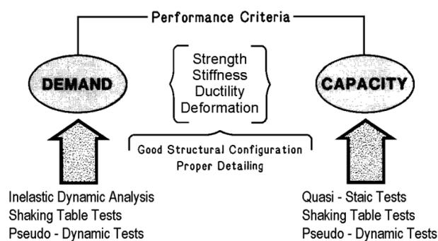
Figure 1. Components of and considerations in earthquake-resistant building design
