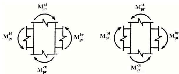
Figure 40. Strong column-weak beam frame requirements.
