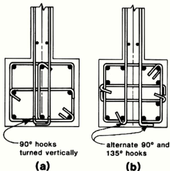
Figure 31. Alternative details for anchorage of horizontal web reinforcement in boundary elements. (54)
