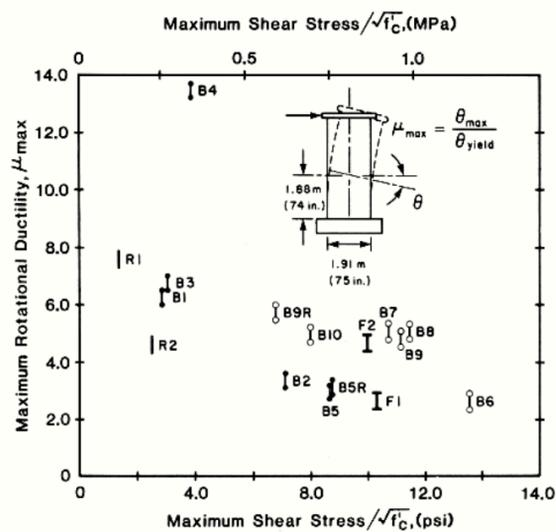
Figure 29. Variation of rotational ductility with maximum average shear stress in PCA isolated wall tests<sup>(51)</sup>.
