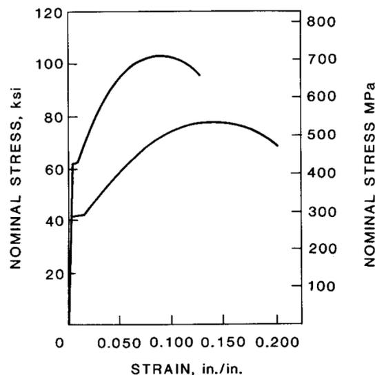
Figure 9. Typical stress-strain curves for ordinary reinforcing steel.
