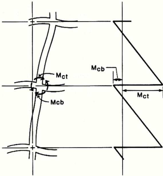
Figure 17. Distribution of bending moments in columns at a joint when the point of inflection is located away from mid-height.
