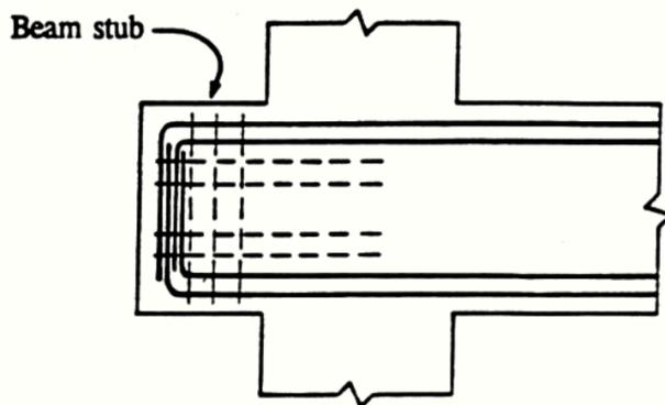
Figure 22. Exterior beam stub for anchoring beam bars
