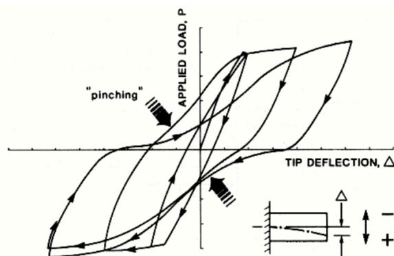
Figure 13. Pinching in load-displacement hysteresis loop due to mainly to sliding shear
