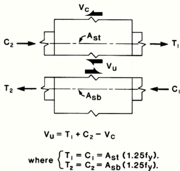
Figure 21. Shear force at mid-height of beam-column joint- ACI Chapter 21 design practice.
