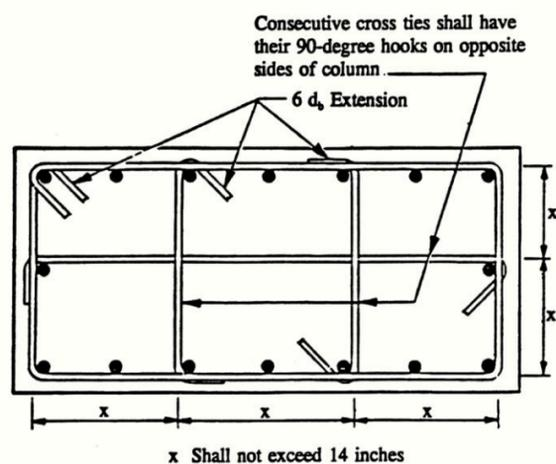
Figure 41. Rectangular transverse reinforcement in columns.
