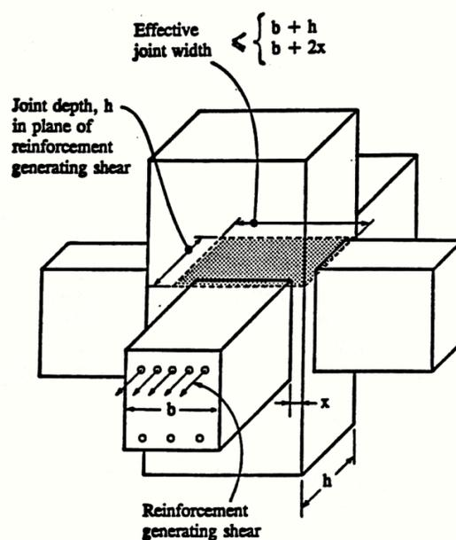
Figure 43. Beam-column panel zone.
