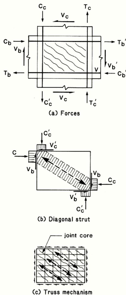
Figure 19. Forces and postulated shear-resisting mechanisms in a typical interior beam-column joint. (Adapted from Ref. 32.) (a) Forces acting on beam-column joint. (b) Diagonal strut mechanism. (c) Truss mechanism.
