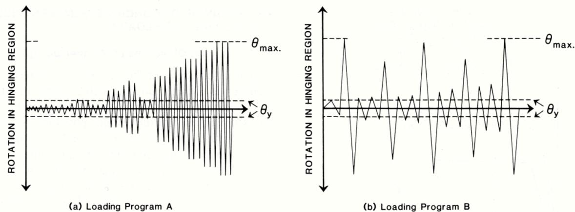
Figure 7 Two types of loading program used in quasi-static tests.
