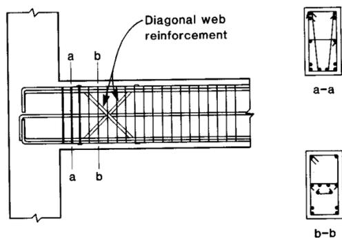
Figure 14. Crossing diagonal web reinforcement in combination with vertical web steel for hinging regions under high shear. (Adapted from Ref. 24)
