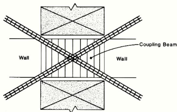
Figure 33. Diagonally reinforced coupling beam.
