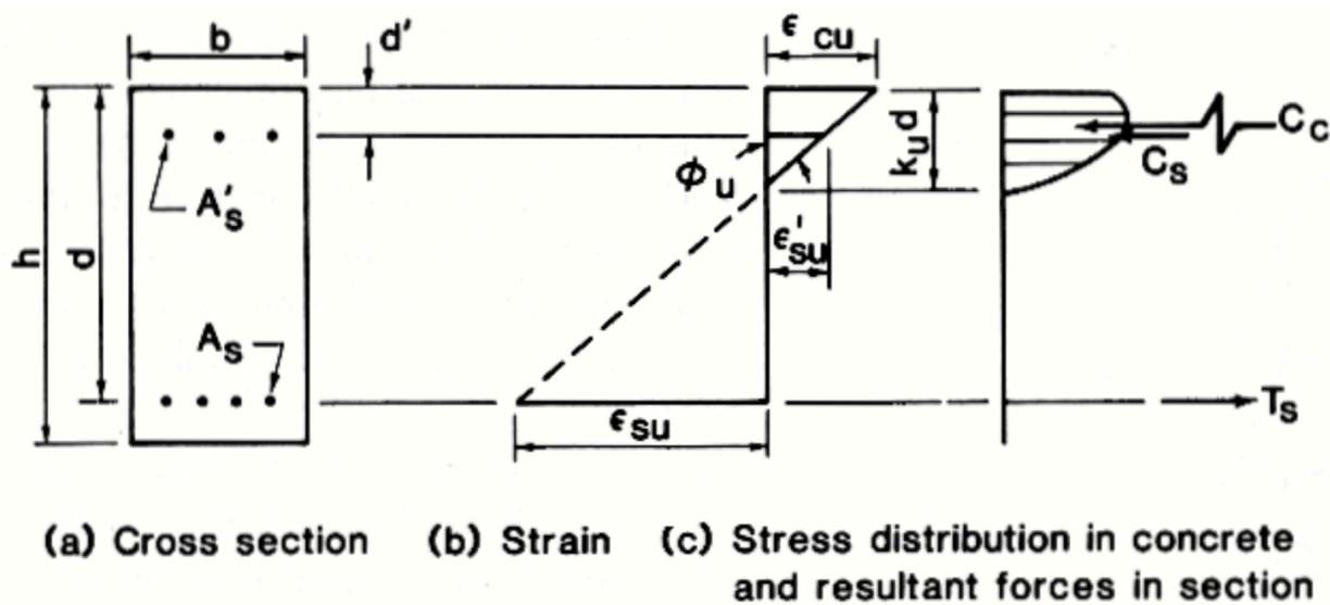
Figure 10. Strains and stresses in a typical reinforced concrete section under flexure at ultimate condition.
