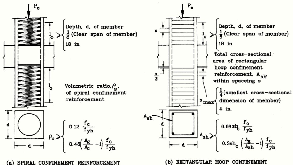
Figure 38. Confinement requirements for column ends.
