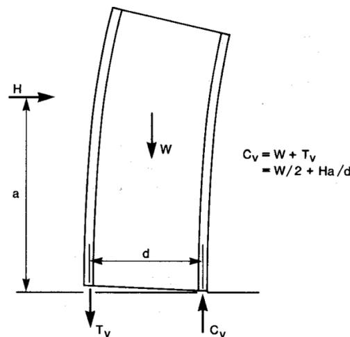
Figure 45. Loading condition assumed for design of boundary elements of structural walls.
