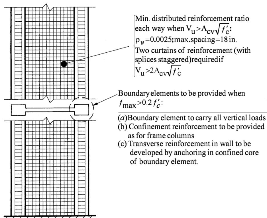
Figure 44. Structural wall design requirements.
