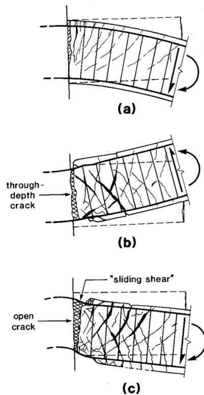
Figure 12. Plastic hinging in beam under high shear. (Adapted from Ref. 31.)
