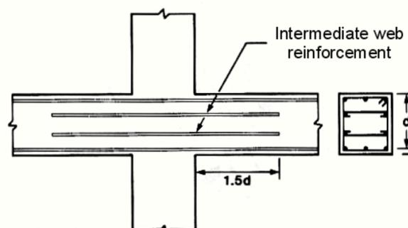
Figure 15. Intermediate longitudinal web reinforcement for hinging regions under moderate levels of shear.
