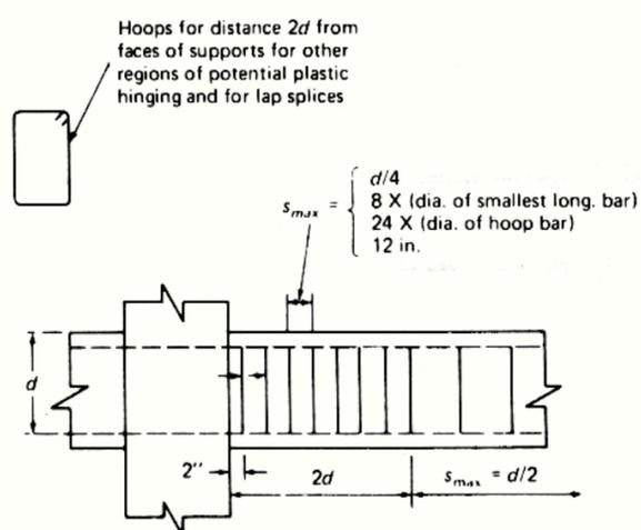
Figure 36. Transverse reinforcement limitations for flexural members. Minimum bar size- #3
